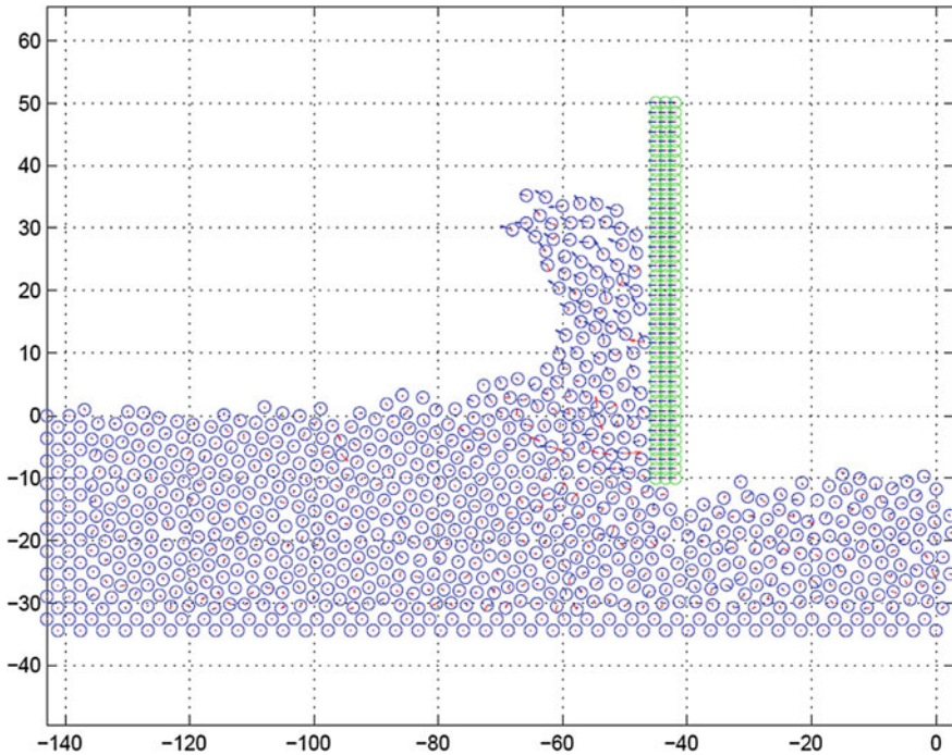
Fig. 5.9 MD simulation of nanometric cutting
