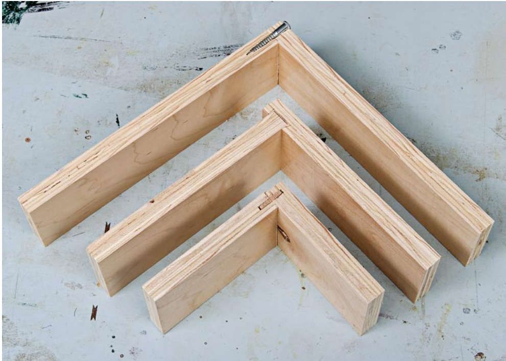
This cross-sectional view shows three commonly used case joints: ready-to-assemble Conformat fastener (top), dado (middle) and spline biscuit (bottom).
