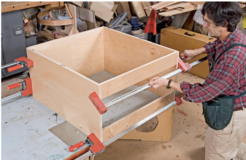
I complete the case assembly by clamping the stretchers between the two side panels.
