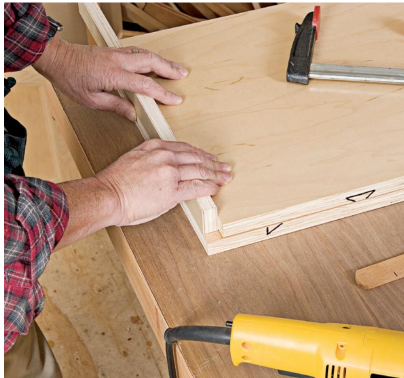
In a similar fashion to the method described for drawer boxes in the last chapter, I use a piece of scrap case material to set the position of the floor panel on the side panel for slotting.
