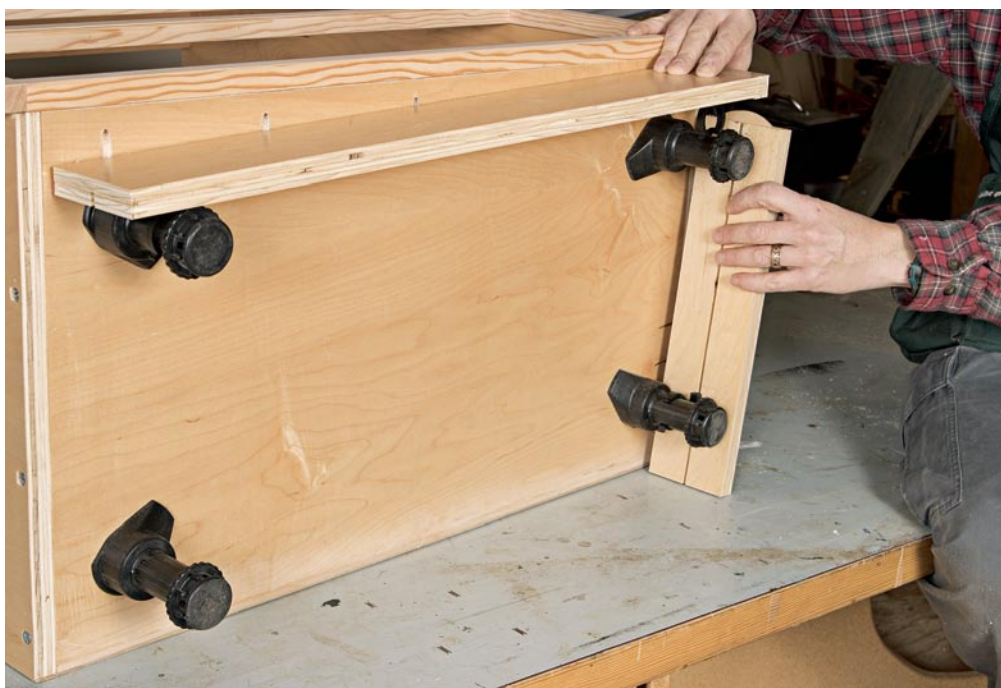
Kick boards fasten to adjustable leg levelers with plastic clips. Note the spline biscuit, which helps keep the corner joint true and secure.
