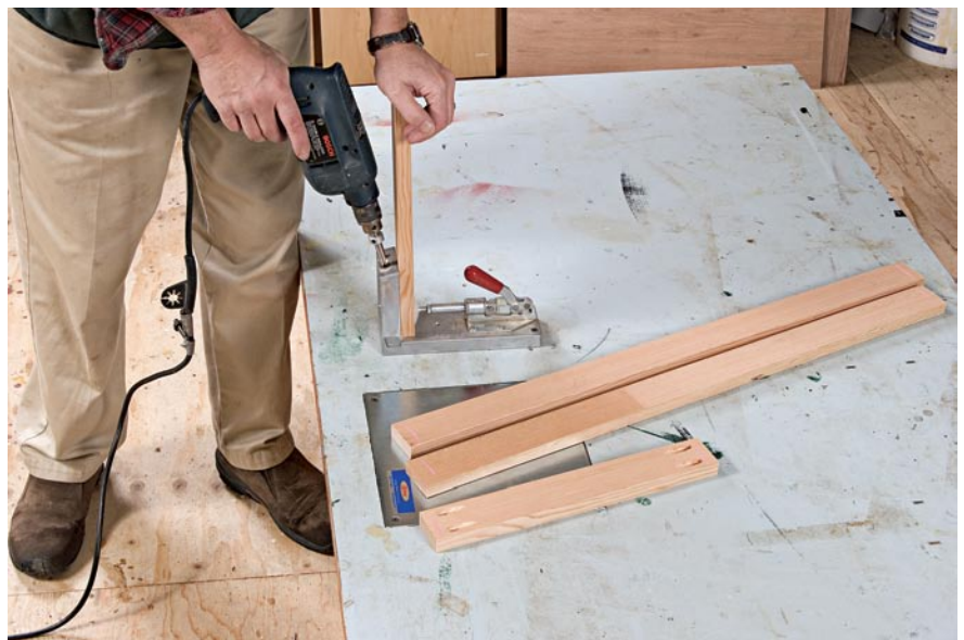
To drill pocket holes in the face-frame stock, I use a proprietary jig to guide the drill bit into the back of the components at each end.
