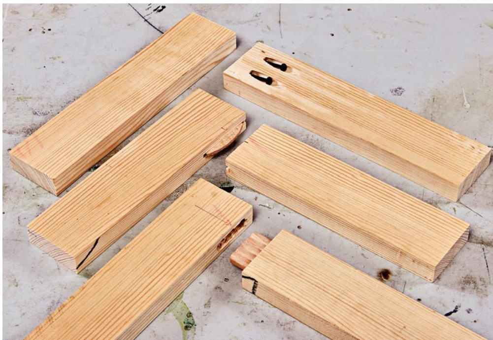
Face frames can be joined quickly and efficiently with pocket-hole screws (top), spline biscuits (middle), or Beadlock tenons (bottom).
