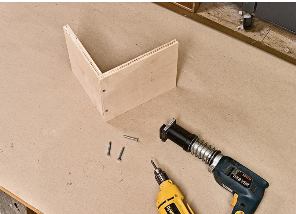
Incredibly strong case fastenings—Confirmat® screws made by Hafele Co. are shown here—are quickly predrilled for use with a proprietary fixture and then installed with a powered screwdriver.
