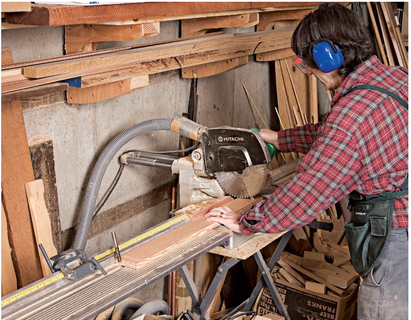
To crosscut stock efficiently with my sliding miter saw, I set it up with side tables and an indexed stop system. (A vacuum hose pulls much of the dust away.)
