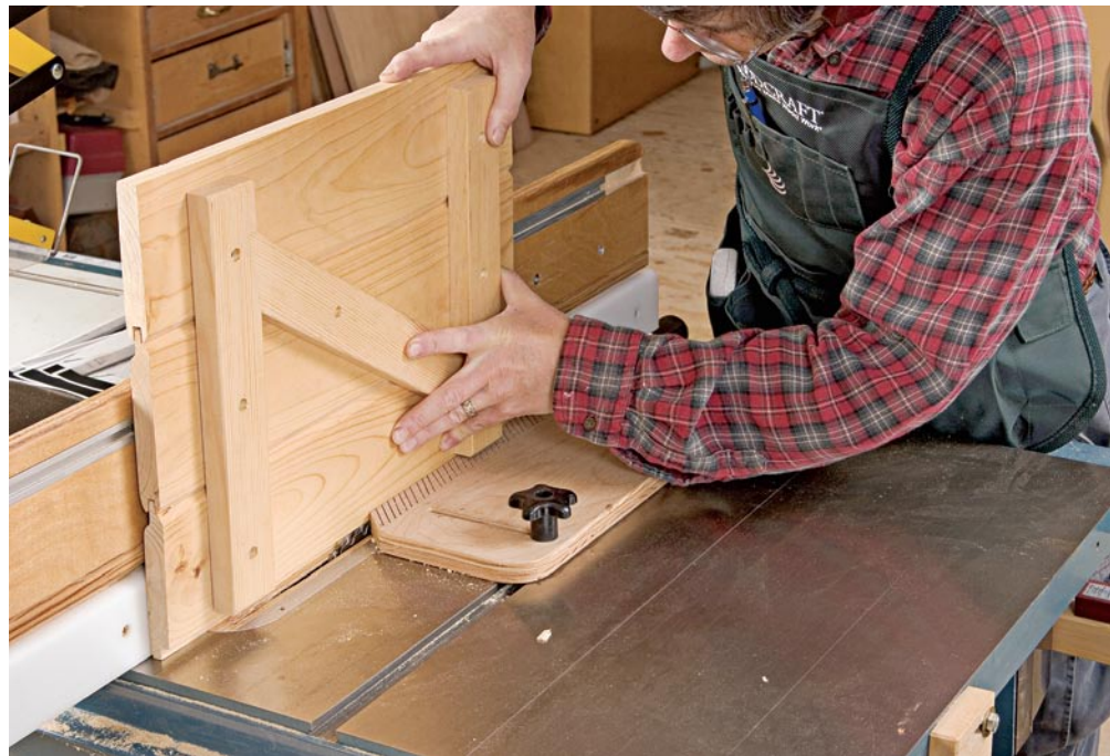
I cut the rabbet for a lipped door on my table saw, using a shopmade featherboard to keep the door tight to the rip fence.
