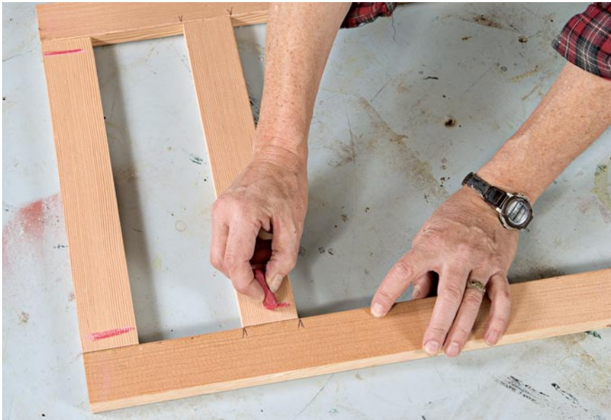
With the face frame placed outside face down on the table, I mark the butt ends of a frame for pocket-screw countersunk holes.
