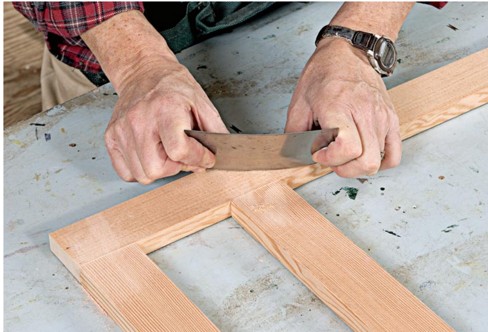
On hardwood, a cabinet scraper makes quick work of flushing the surface of each joint. I follow up with 180-grit sandpaper on a random-orbit sander.
