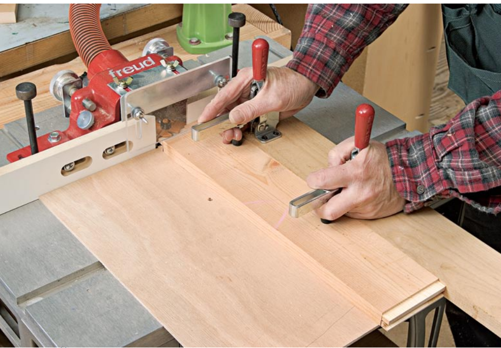
To make the cope cuts at the ends of each rail, I use a shop-made carriage to guide the stock past the coping cutter. (photo © Craig Wester)
