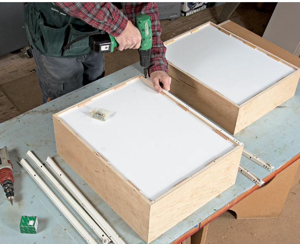
To make hardware installation go quickly, I separate the drawer runners into right- and left-hand pieces, placing them to the appropriate side of the assembly area. Then I install them to the each drawer box.
