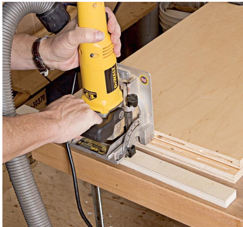
I stand the joiner on its face to make matching slots in the side panel.
