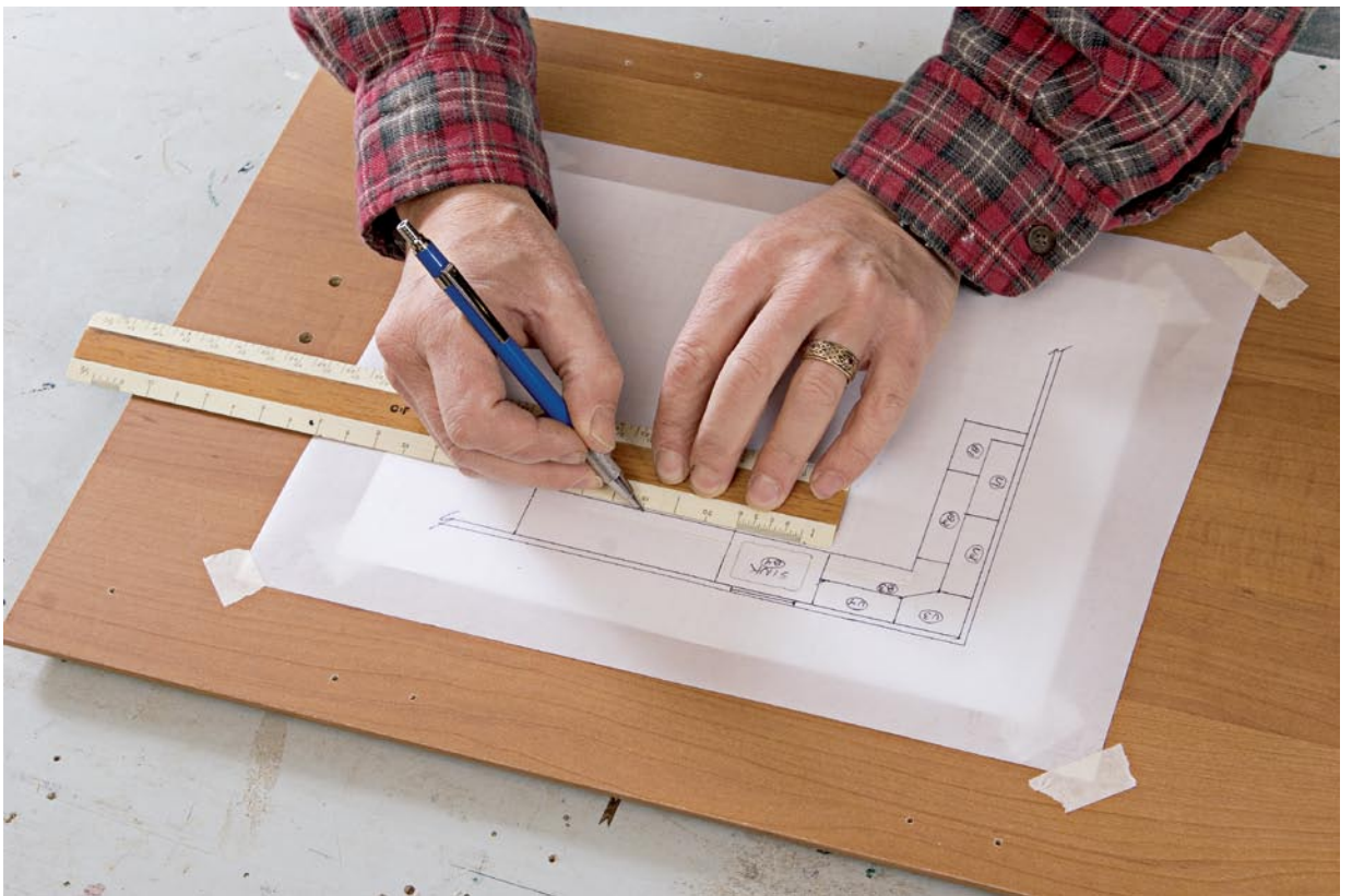
Satisfied with the full-scale layout, I next create floor and elevation views (at 1-in. = 1-ft. scale) on translucent vellum paper taped over a grid sheet.
