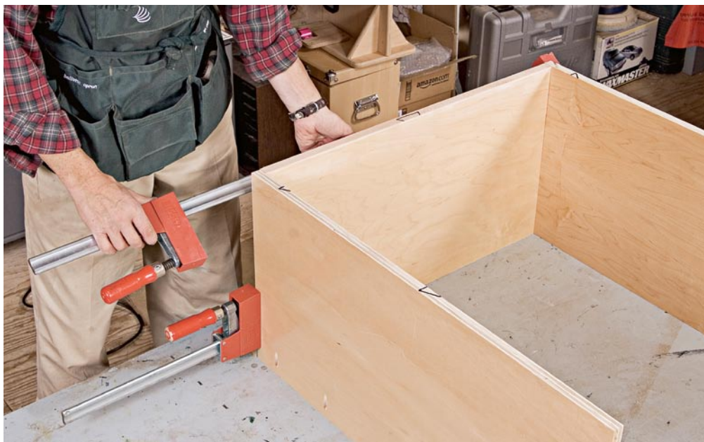
After fastening the first corner together, I then clamp the second side panel to the floor panel.
