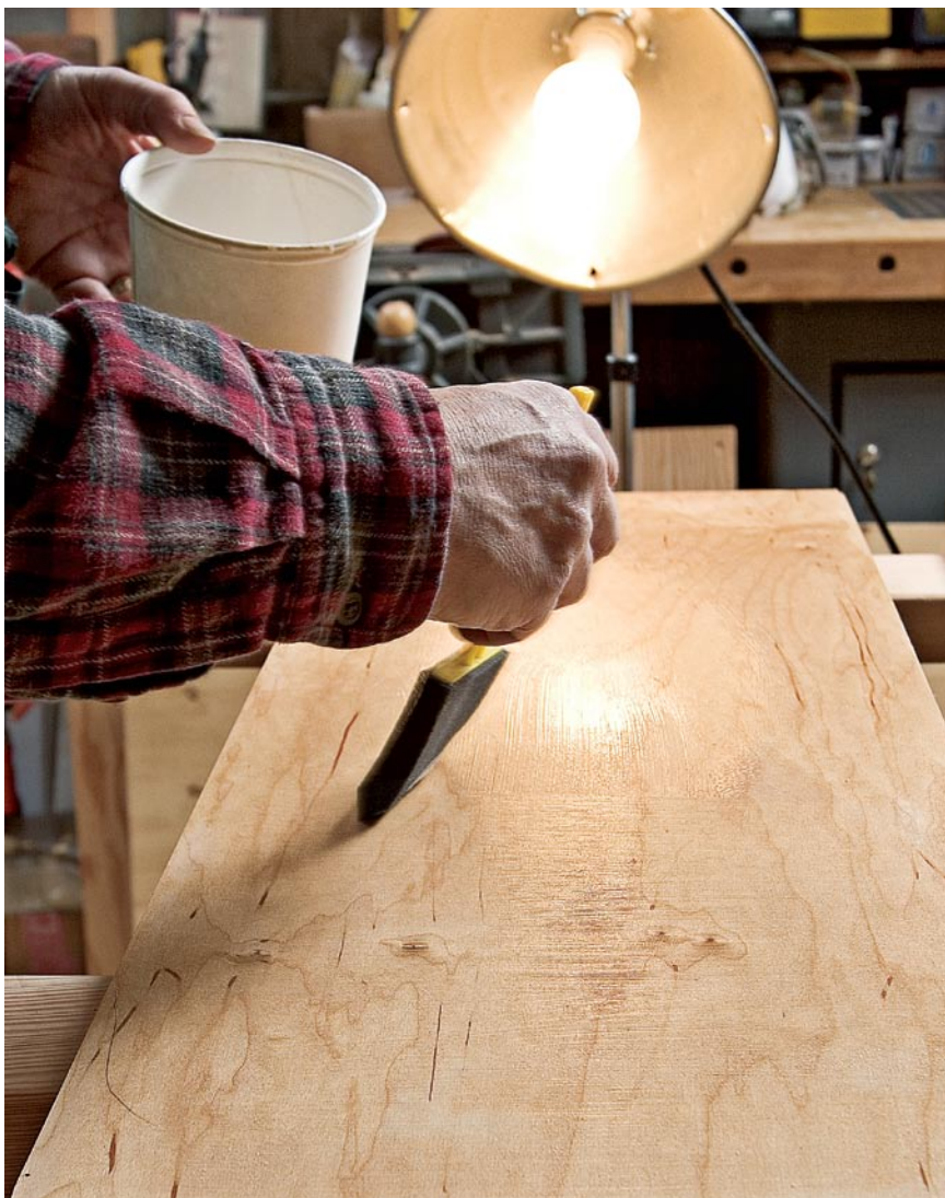
Setting up a light at a low angle makes it easy to detect dust, heavy brushstrokes or missed spots in the finish.
