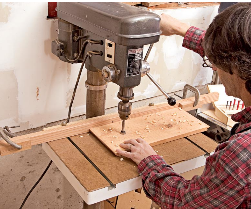
A stopped fence system on the drill press makes quick, accurate work of drilling the back of the drawer faces for their attachment fittings.
