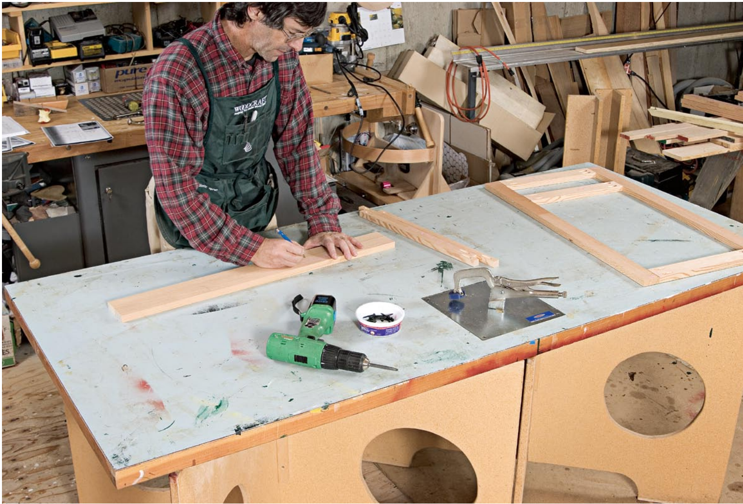
To make a sturdy, yet temporary, work table, I surface an old solid-core door with laminate and support it on knock-down lifts.
