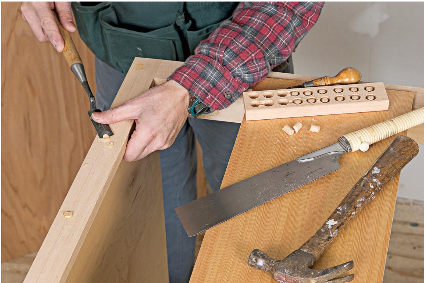
I use a specialized Japanese goose-neck chisel to trim the bung flush with a series of incremental slices. Any sharp chisel, however, will do.
