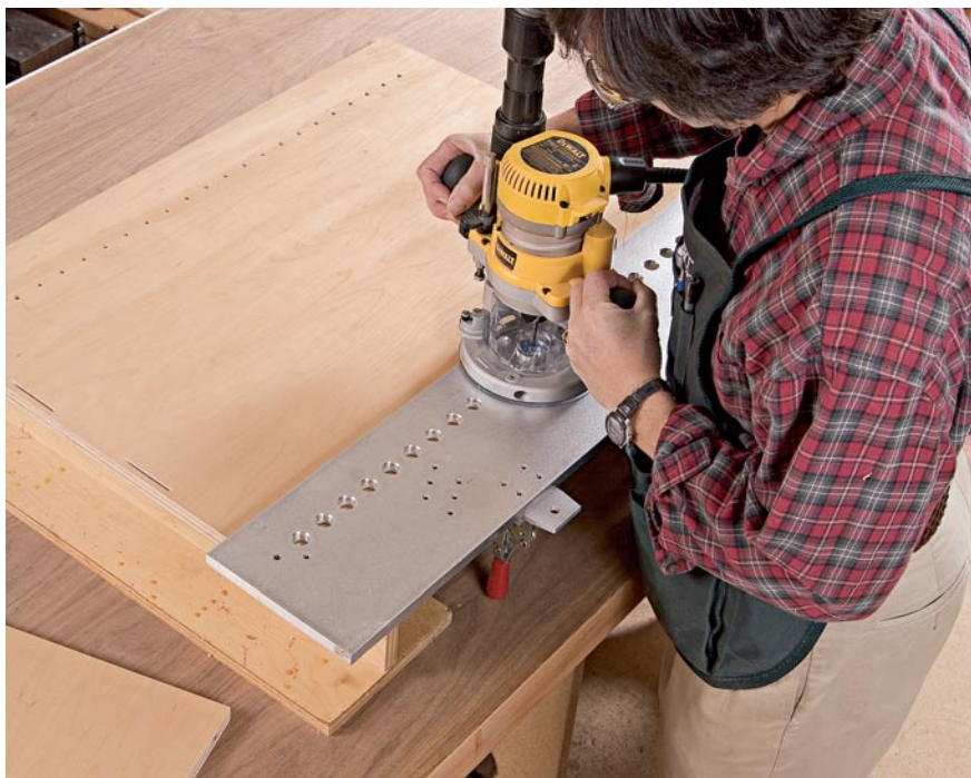
Using a commercially made jig by MEG® Products and a plunge router I can quickly create a precisely spaced line of holes for shelf clips.
