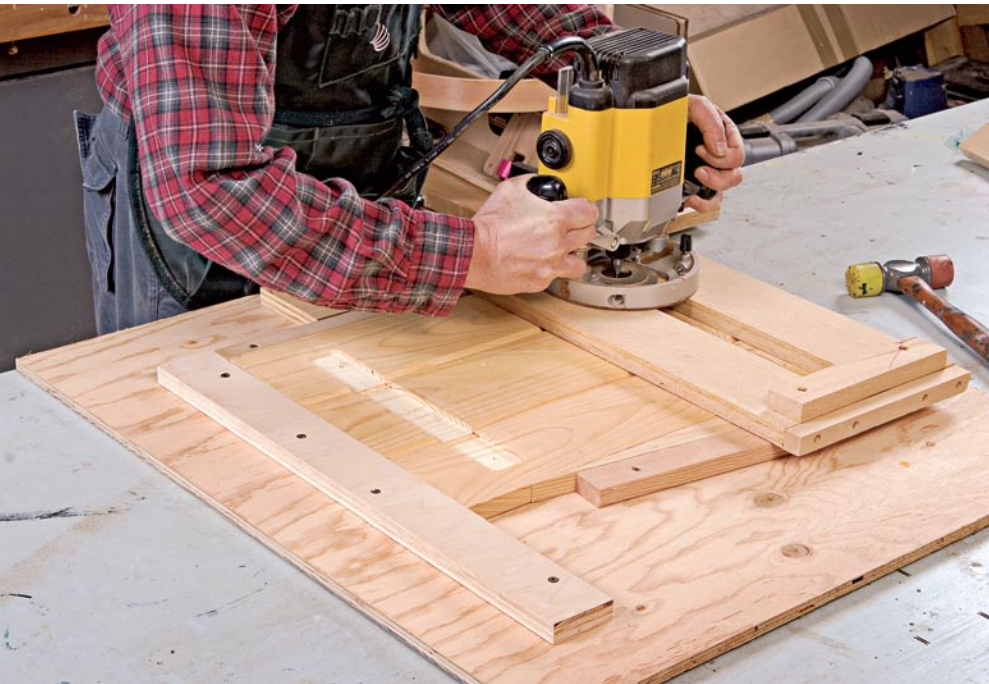
I rout the dados for the door battens using a shopmade router guide.
