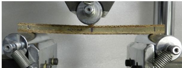
Figure 4. Sandwich sample mounted on flexural test set-up
