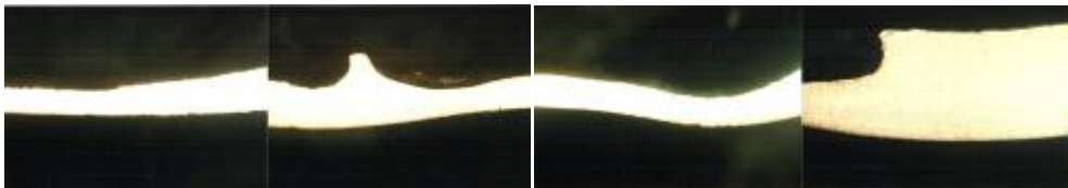
Figure 11. Macrograph of 5-7 o'clock position showing the absence of ERW.
