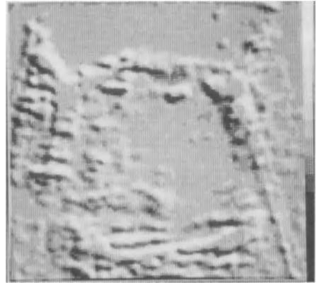
Fig. 7. Phase-dependent filtering (pseudo-three-dimensional). By this transformation, small intensity modulations can better accentuated. The apparent angle of "incidence of light" can be varied, thus sharpening the contrast (filtered version of Fig. 3 a).
