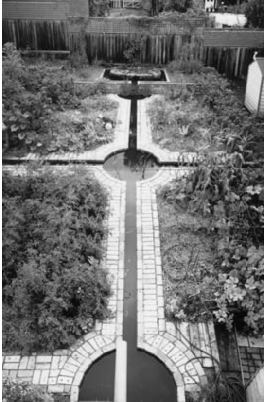
Fig. 4.5 A rainwater collection system in a suburban backyard becomes a water feature as well as an irrigation channel. Photograph by Andrew Wood.
