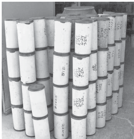
Standard capped cylinders ready for testing.
