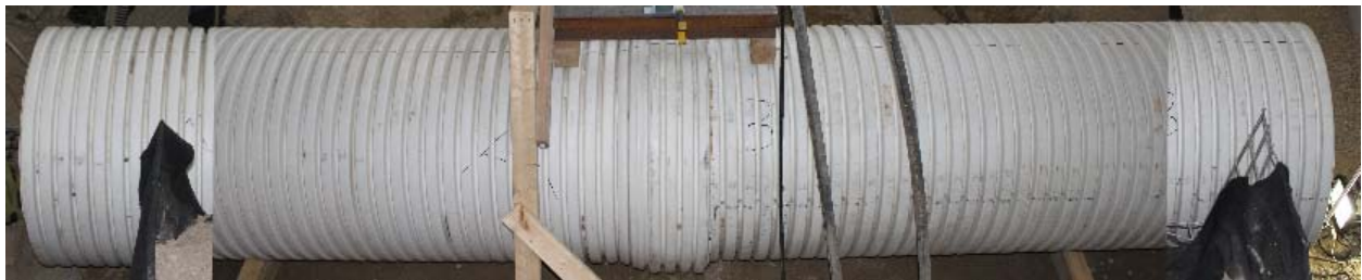
d. 36 inch (914mm) diameter PVC pipe with gasketed bell and spigot joint
