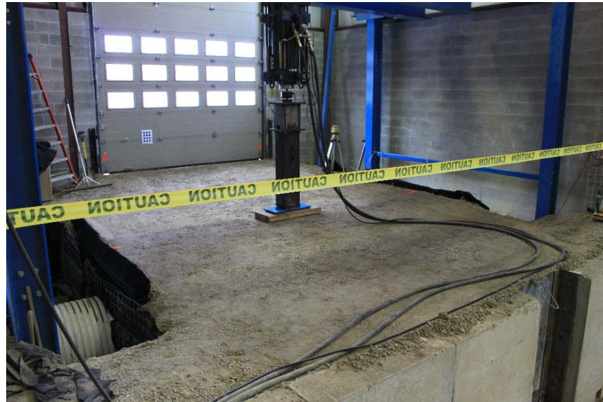
Figure C.90. Ultimate limit state test configuration of the 36 in. (915mm) diameter PVC pipe.
