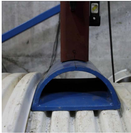
Figure H.8 End of loading frame on timber support. Figure H.9 Curved load plate and column.
