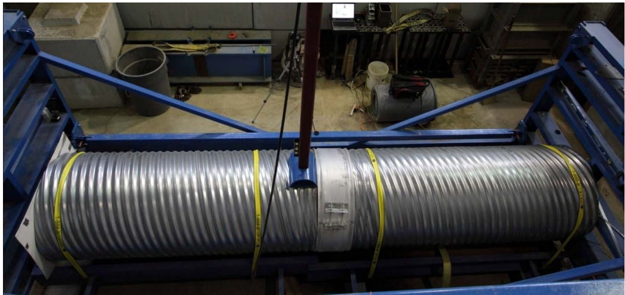
b. Configuration of the shear test on the CSP; hinges are removed to disconnect the frames and the left end of the left frame sits on a wooden support; shear force is applied immediately left of the joint.
