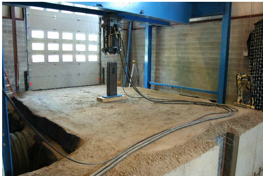
Figure C.91. Ultimate limit state test configuration of the 60 in. (1525mm) diameter HDPE pipe.
