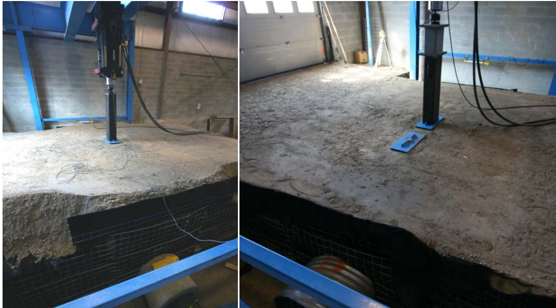
a. 24 in. (0.6 m) RCP at 4 ft (1.2 m) cover b. 36 in. (0.9 m) CSP at 2 ft (0.6 m) cover Figure 4. Live load testing of two of the jointed culvert systems tested in the laboratory.
