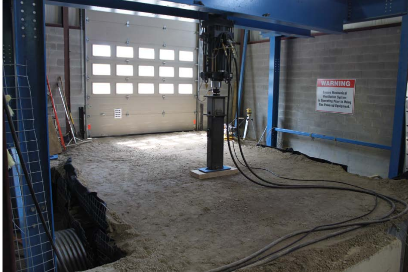
Figure C.58. Configuration of the ultimate limit state test for the 36 in. (915mm) diameter corrugated steel pipe; size of the loading pad was increased to prevent bearing failure.
