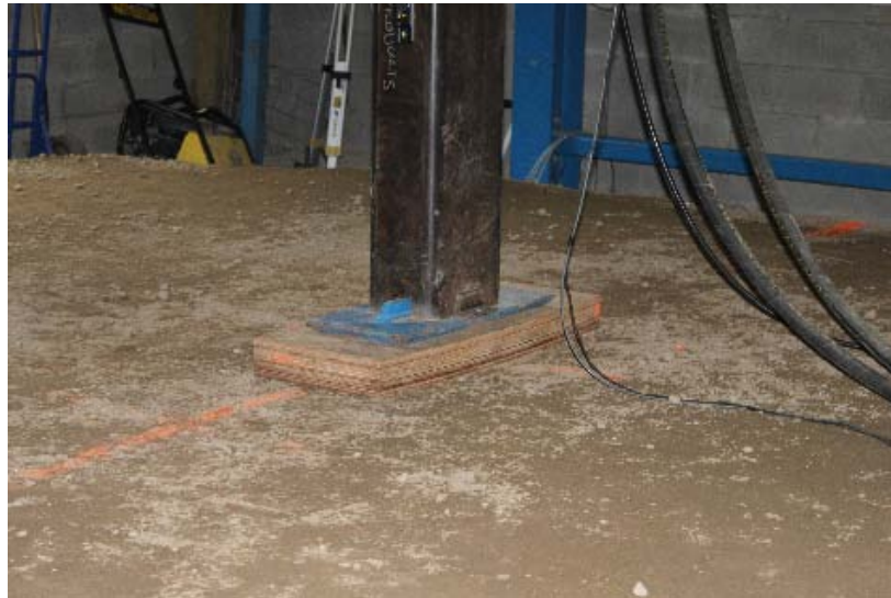
Figure C.22. Increased size of the loading pad employed in the ultimate limit test of the reinforced concrete pipes (to prevent or delay bearing capacity failure under the loading pad).
