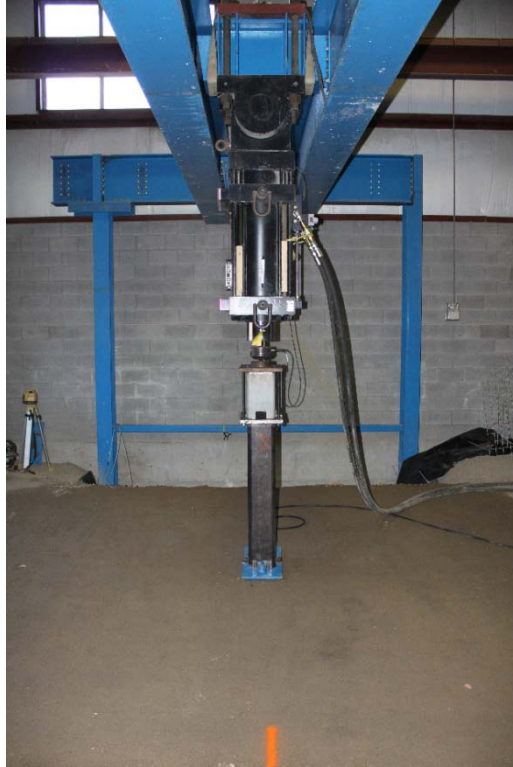
Figure C.78. Steel loading plate, loading column and 2000 kN (220US ton) capacity actuator.
