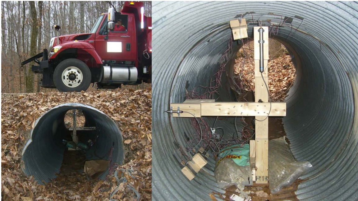
a) Loading on the culvert
