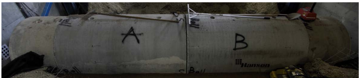
e. 48 inch (1220mm) diameter reinforced concrete pipe with unsealed bell and spigot joint
