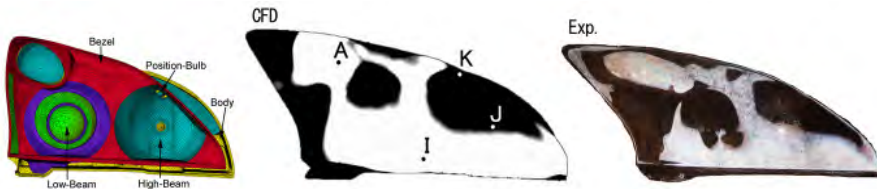
Fig. 6. Moisture and natural convection simulation inside an headlamp: Front view of the numerical mesh and the moisture condensation after 20 min (reprinted with permission from SAE Paper 2005-01-1449 ©2005 SAE International).
