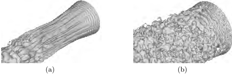
Fig. 7. Instantaneous density contours, (a) shear layer between primary and secondary jet, (b) shear layer between secondary jet and surrounding fluid. (Courtesy of N. Andersson et al. [24]).
