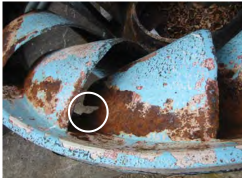
Fig. 7. Cavitation erosion at the blade's leading edge.
