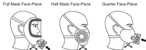
Figure 28-1. Types of Tight-Fitting Respirators by Face-Piece. Adapted from: Bollinger NJ, Schultz RH. NIOSH guide to industrial respiratory protection. National Institute of Occupational Safety and Health. Washington DC, September 1, 1987 Publication No. 87-116. Web site: http://www.cdc.gov/niosh/87-116.html . Accessed October 22, 2003.
