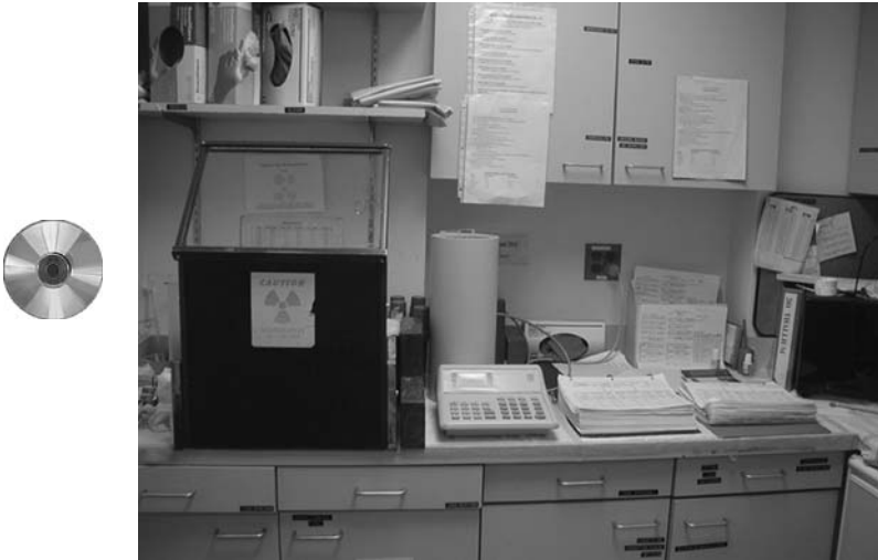
Fig. 1-3. Interior of the radiopharmacy, also known as hot lab. On the left is the lead-shielded work area. In the middle is the dose calibrator. On the right are the logbooks for recording the use of radioisotopes.
