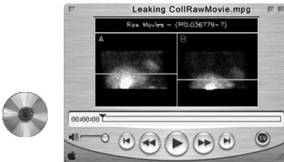
Fig. 16-53. Rotating stress (A) and rest (B) planar projection images. During the rotation of the stress images a bright “glow” appears on the top of the images in the anterior positions. This is most likely due to “leaking” radioactivity from outside the field of view between the mounted collimator and the gamma camera detector head. The technologist must investigate the cause of this artifact by surveying the patient’s gown, neck and arms for contamination or extravasation of injected dose. It is also possible that the collimator is not mounted correctly on the camera head. This is potentially dangerous because the collimator could fall off and injure the patient. If the collimator is mounted correctly, one can purchase lead guards that cover the slit between the collimator and camera, and this will avoid this artifact from recurring. (movie).
