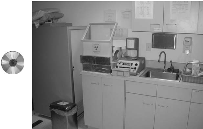
Fig. 21-3. Hot-lab area in Chest Pain Center. The lead-shielded working area and the dose calibrator fit on the counter top next to the zinc. Note wastebasket for radioactive waste.
