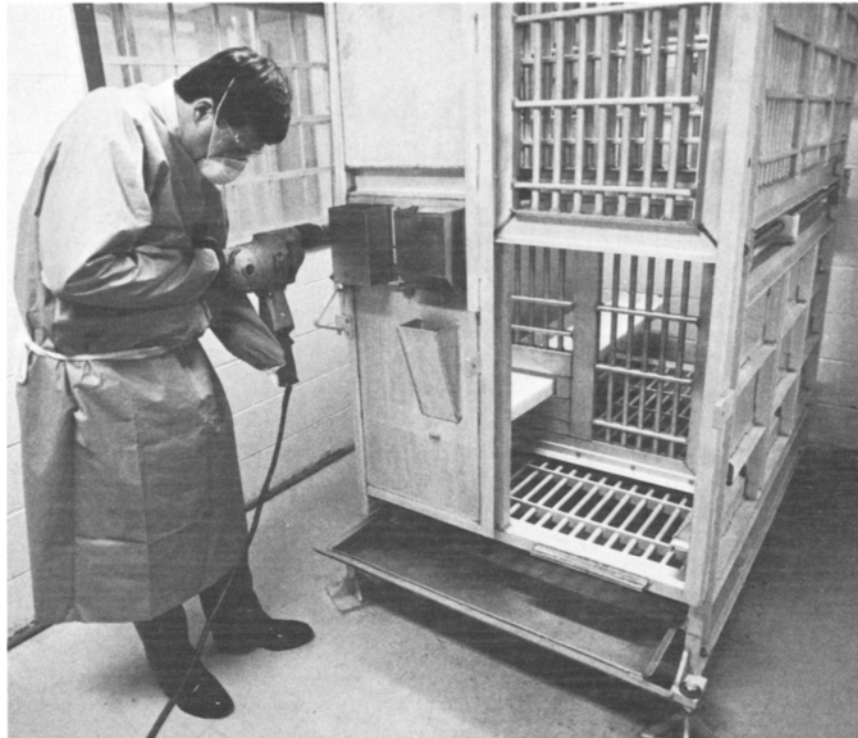
Fig. C.5 A squeeze-back cage with an electrically operated screw mechanism.
