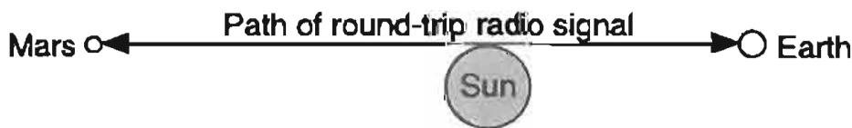
Figure 1 Diagram, not to scale, of the path of radio signals that graze the surface of Sun on their round-trip between tracking stations on Earth, right, and a Viking lander on the surface of Mars, left. Note: The path bends near Sun, but by an angle less than 2 seconds of arc, far too small to show on this or later diagrams.
