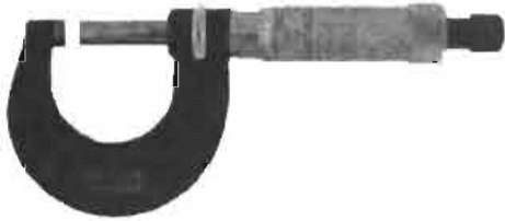
Figure 8 A micrometer caliper, used to measure small distances, such as the thickness of metal sheet. A calibrated screw on the right meters the gap between cylinders at the left.
