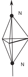
Figure 7.1 The ammonia molecule with the two equivalent equilibrium positions of the nitrogen atom
