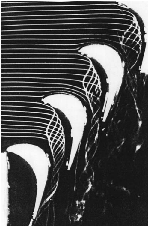
Figure 9.13: Visualization of secondary flow near the endwall of a turbine blade cascade (Gostelow, 1984).
