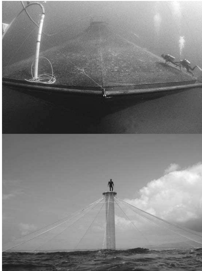
Fig. 8.3. Submersible, semirigid net cages for use in deep water. The top photograph is a 3,000-m 3 cage deployed 2 km off Ewa Beach, Oahu, used to raised Pacific threadfin ( Polydactylus sexfilis ). Threadfin, locally called moi, are a highly esteemed fish with deep cultural significance in Hawaii. The bottom photograph is a 3,000-m 3 submersible cage deployed 1.5 km off the Kona Coast of Hawaii. The cage is used to grow sashimi-grade Hawaiian yellowtail ( Seriola rivoliana , also called Almaco jack). The cage is normally submerged, as in the top photograph, but it is floated above water for cleaning and maintenance. Photographs courtesy of OceanSpar LLC.
