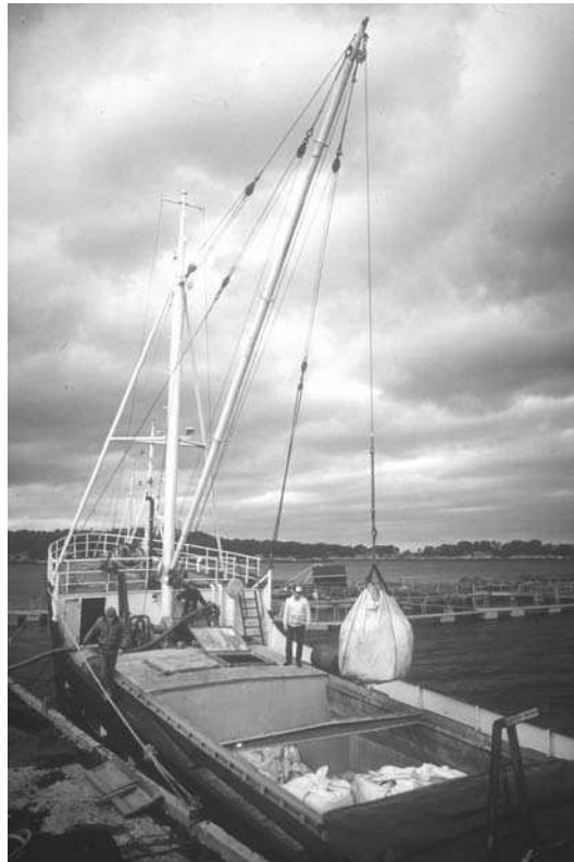
Fig. 8.6. Off-loading feed from a work boat to a net-pen facility in Maine. Feed transport and handling must be conducted carefully to minimize generating “fines” by abrasion of feed pellets.
