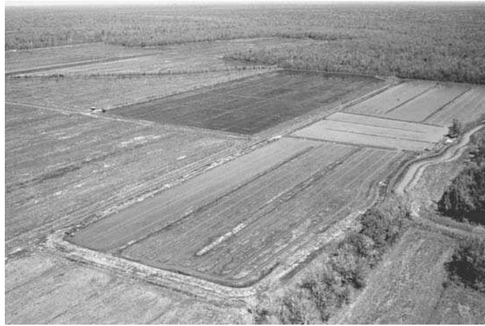
Fig. 6.4. Crayfish ponds in Louisiana. The pond in the foreground is approximately 12 ha. Note earthen baffles that direct water from the well (lower-left corner) to the outlet (upper-right corner) of the pond in the foreground. Photograph courtesy of the LSU AgCenter.
