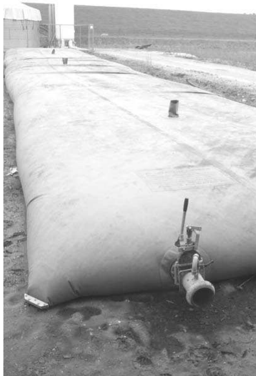
Fig. 10.13. A large, impermeable plastic storage bag with gas vents through the top of the bag offers a lower initial fixed cost option to fish manure storage.
