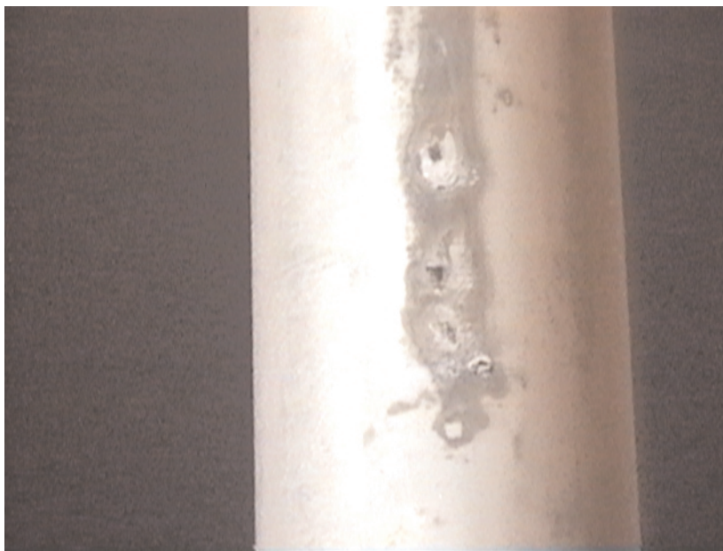
Figure 4.2 Most of DOE's spent nuclear fuel is stored underwater to provide cooling and radiation shielding. A variety of corrosion processes, such as the pitting shown here, are degrading many of the fuels. Source: DOE National Spent Fuel Program.
