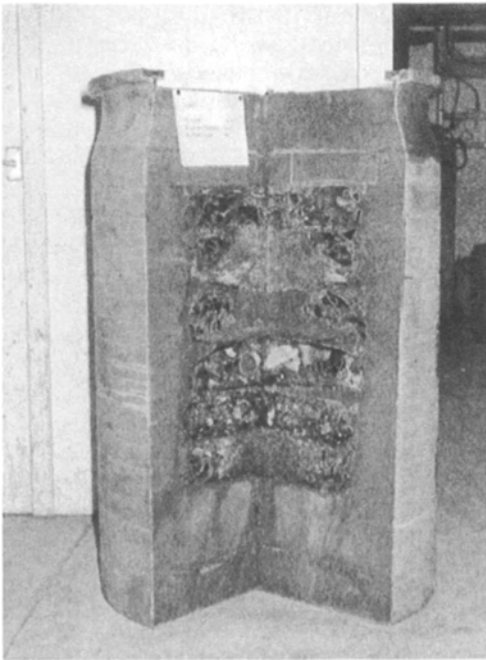
Figure 20-7. Cross-section of Compacted PCM Pucks in Standard 500l Stainless Steel Container (Photograph Courtesy of BNFL Magnox).
