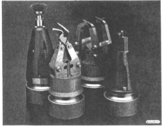
Figure 9-4. Some of the Tools Developed for Remote Weld Sampling (Photograph courtesy Schilling).
