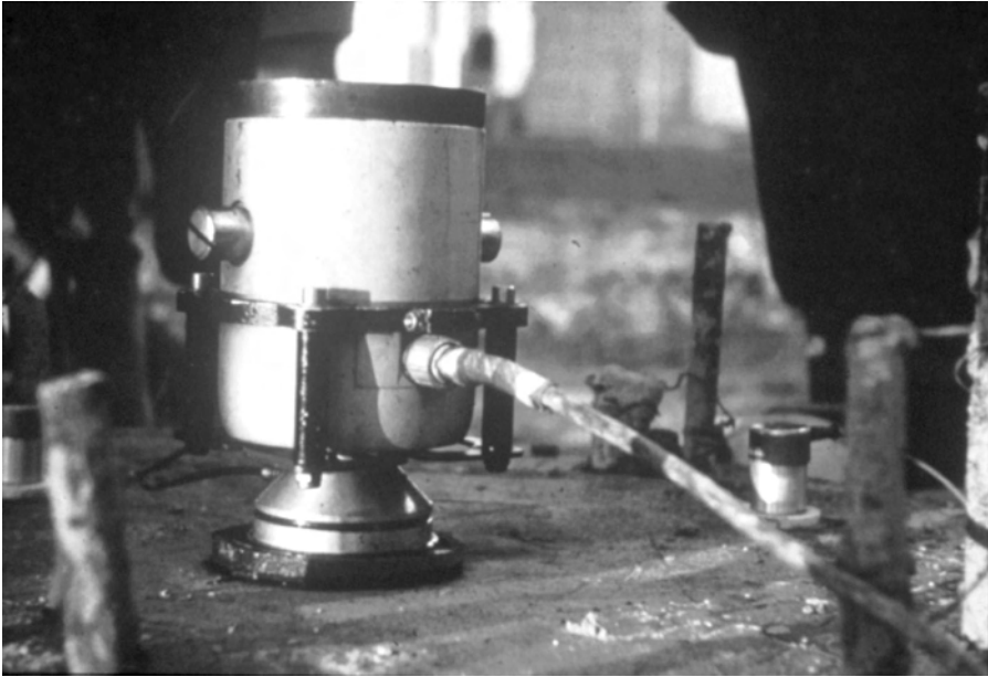
Figure 8.1 Instrumentation set-up for the Vibration test on a drilled shaft
