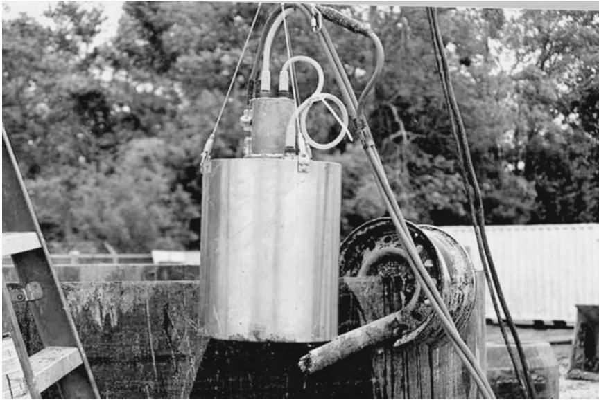
Figure 4.5 'Mini-SID' ready for deployment down a shaft. Reproduced by permission of Applied Foundation Testing, Inc., Florida, USA
