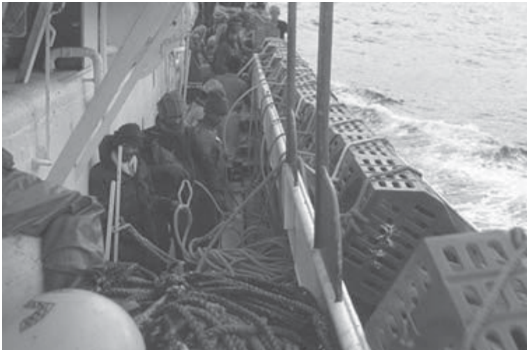
Fig. 12.9 Long-line system with top-entry plastic traps used in the fisheries for Palinurus gilchristi and P. delagoae .
