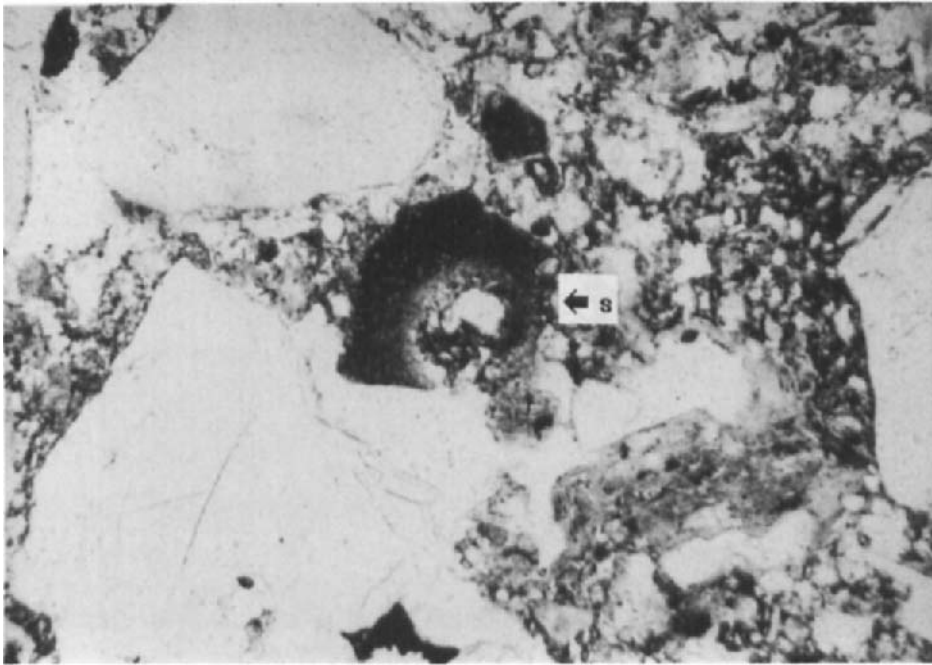
Fig. 9. Micrograph of thin section from a duric horizon of a soil from near Yeoval, New South Wales, Australia showing a channel filled with amorphous silica (s); PPL; FW 15.8 mm.
