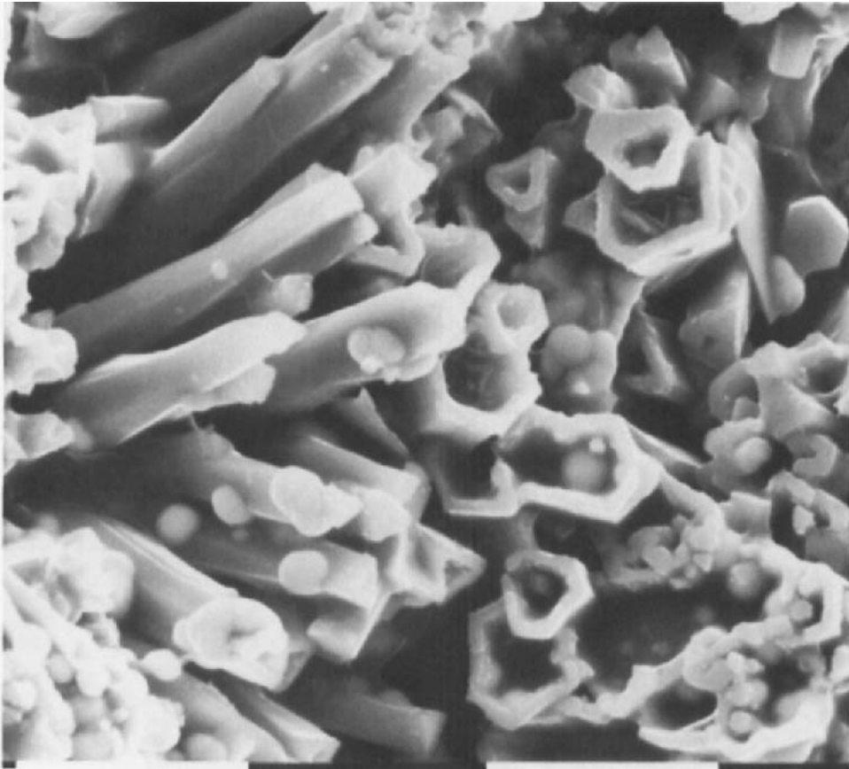
Fig. 4. Scanning electron photomicrograph of a Mn-rich area from 10 m depth in the M2 core showing rods of lithiophorite ((\text{Al}, \text{Li}) \text{MnO}_2 (\text{OH})_2) crystals and balls of intimately mixed Ce/U oxides. Scale bar is in 10 \mu\text{m} sections.
