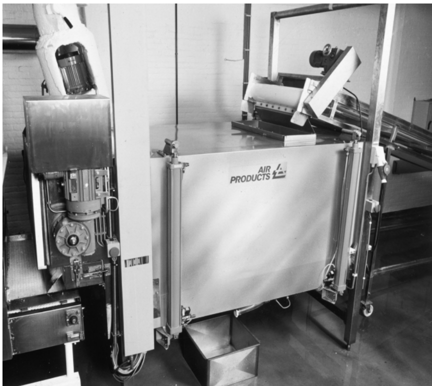
Fig. 9.16 Immersion freezers use a bath of liquid nitrogen to give rapid freezing of prawns and other IQF products. This Air Products Cryo-Dip has a throughput of 2–5 t/h.
