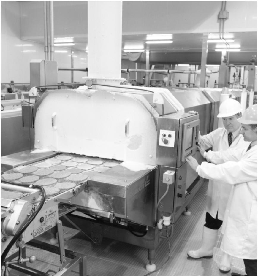
Fig. 9.11 Cryogenic tunnel freezers are similar to mechanical refrigeration blast freezers, but with spray nozzles for liquid nitrogen or liquid carbon dioxide instead of evaporator coils. This Air Products Cryo-Quick VT freezer is an unusual design. Fans beneath the belt reduce liquid nitrogen consumption, while a vortex-inducing curved upper section gives vertical gas velocities and hence rapid freezing.
