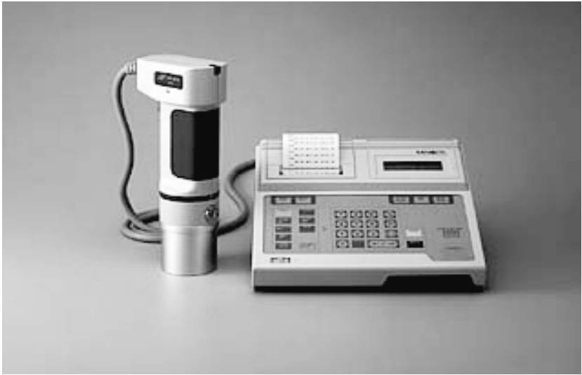
Fig. 3.9 Minolta Chroma Meter. (Source: courtesy of Minolta Ltd, Japan.)
