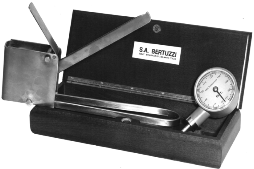
Fig. 3.7 Portable and laboratory dynamometer for measuring the consistency of peas. (Source: courtesy of Bertuzzi SA, Italy.)
