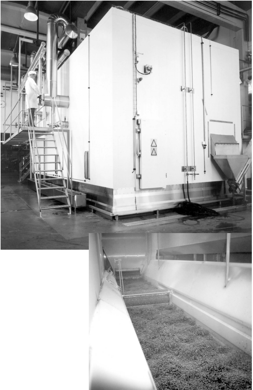
Fig. 9.18 The Frigoscandia FLoFREEZE M is a fluidised-bed mechanical refrigeration freezer with two freezing zones. Inset: peas are a typical application of IQF freezing in a fluidised bed.
