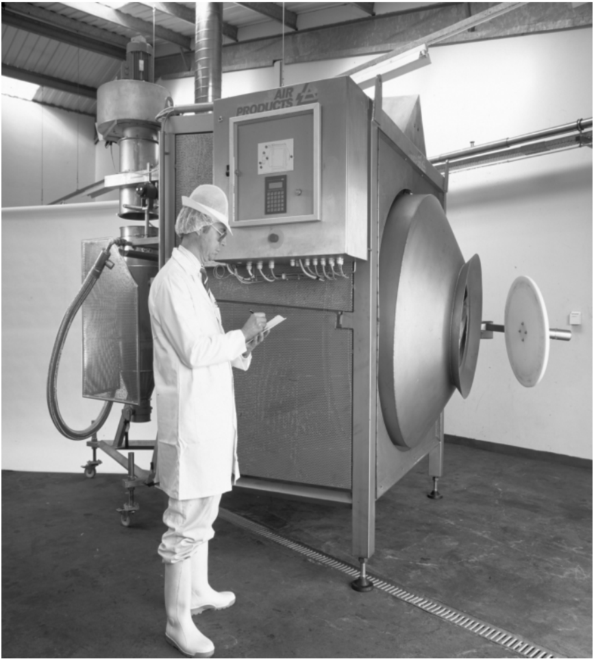
Fig. 9.19 A tumbling freezer such as this Air Products Cryo-Tumbler is a batch device ideal for coating IQF products with sauces or breadcrumbs. A unit measuring 3.1 m high, 3.5 m long and 2.9 m wide has a capacity of 850 kg of product. The continuous version, known as a rotary tunnel freezer, works in a similar way but is longer (6–12 m) and smaller in diameter (800–1200 mm).
