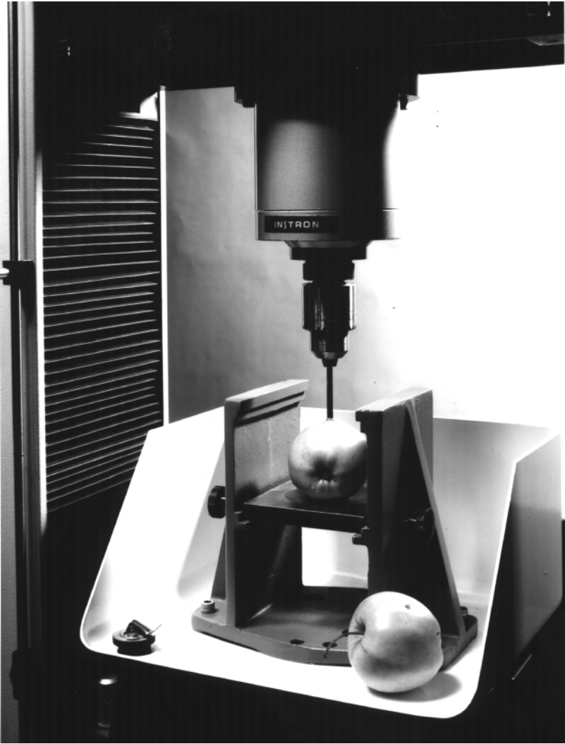
Fig. 3.8 Instron Universal Testing Machine. (Source: courtesy of Instron Ltd, UK.)
