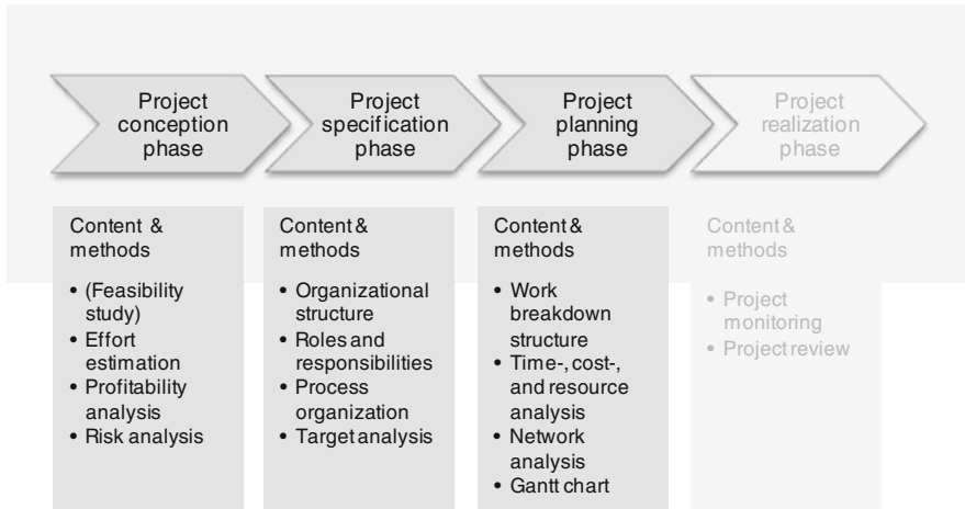
Fig. 12.2 Phases, content, and methods of the project life cycle (Zimmermann et al. 2010)
