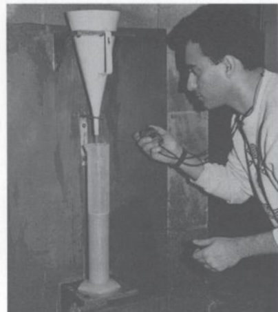
Fig. 7.8 Determination of the Marsh cone flow time (courtesy of M.Baalbaki).
