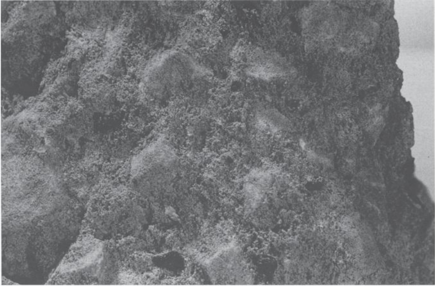
Fig. 5.1 Failure surface of a usual concrete.
