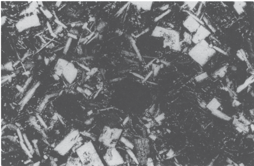
Fig. 6.39 Air-cooled or crystallized slag under polarized light in an optical microscope. The white prismatic crystals are melilite.
