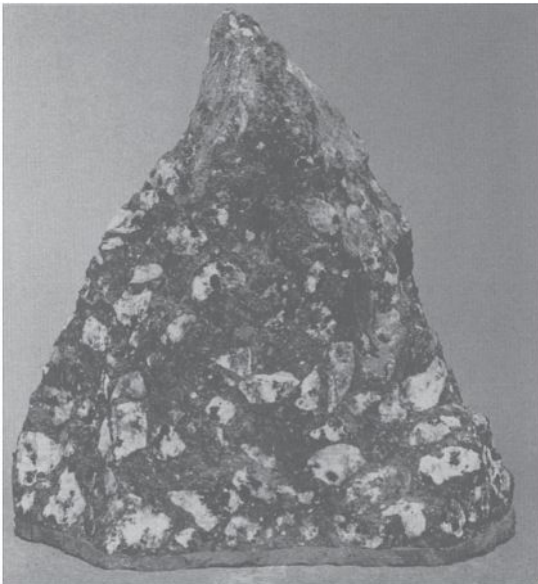
Fig. 5.2 Failure surface of concrete containing a weak coarse aggregate. The failure planes have propagated through the coarse aggregate particles.
