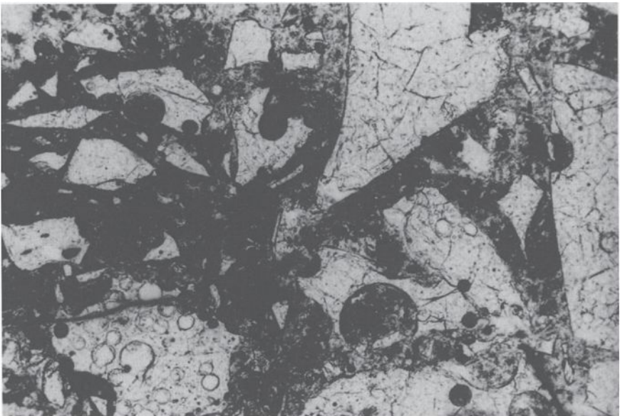
Fig. 6.41 Vitreous slag particles (in white). Note the shape of the slag particles and their porous aspect due to quenching in water. The totally vitreous particles of slag denote that the temperature of this slag was high when it was quenched (such slag is sometimes referred to as 'hot slag').
