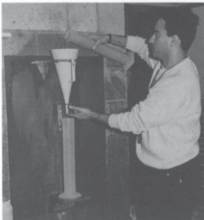
Fig. 7.8 Determination of the Marsh cone flow time (courtesy of M.Baalbaki).
