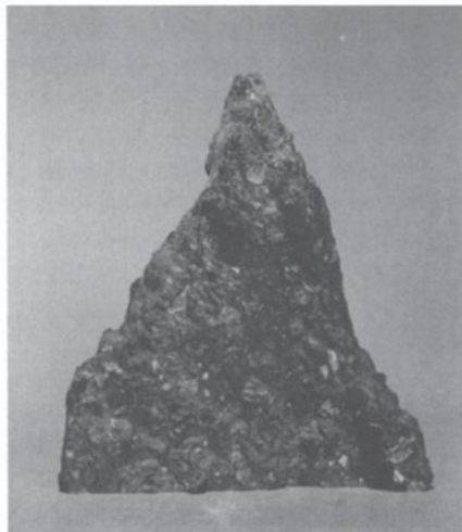
Fig. 15.5 Typical conical failures: (a) the coarse aggregates have been crushed; (b) debonding of the coarse particles of the gravel; (c) a 150 MPa failure.
