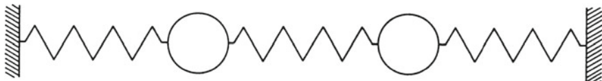
Fig. 1.11 Two coupled one-dimensional oscillators between two fixed walls. All three spring constants are equal
