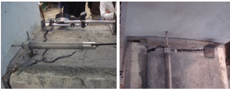
Fig. 5. Splice regions under tension. Element CVP-2B (left), element CVP-1A (right)
