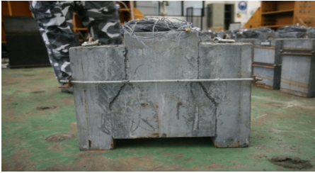
Fig. 8. Failure of UHPFRC precast joint (Cast-in-place joint)
