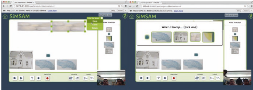
Fig. 3.2 The SiMSAM modeling environment interface, illustrated the program-by-demonstration and menu of options command features. Shown on the left , program-by-demonstration is using the “Move” command in one of the menus. The user moves the object some distance, and the program records the relative distance and position of that motion as a translation rule governing that object’s motion when the simulation is run. Shown on the right , interactions between objects are programmed using the “When I bump...” command, whereby the user selects the two objects to consider in the interaction and sets the rules for how they behave once they come in contact with one another
