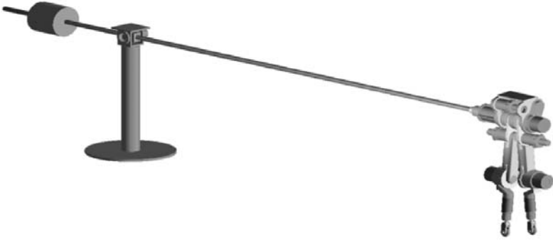
Figure 2.2. RABBIT's setup, which includes a boom to constrain the robot's path to a circle. The boom is attached at the robot's hip, via a revolute joint. The boom only provides lateral stabilization; it does not prevent the robot from falling forward, backward, or down. The counter balance can be used to offset the weight of the lateral stabilization bar or to modify the effective gravitational field. Not shown are the dSPACE module and power electronics that are mounted on top of the central tower.
