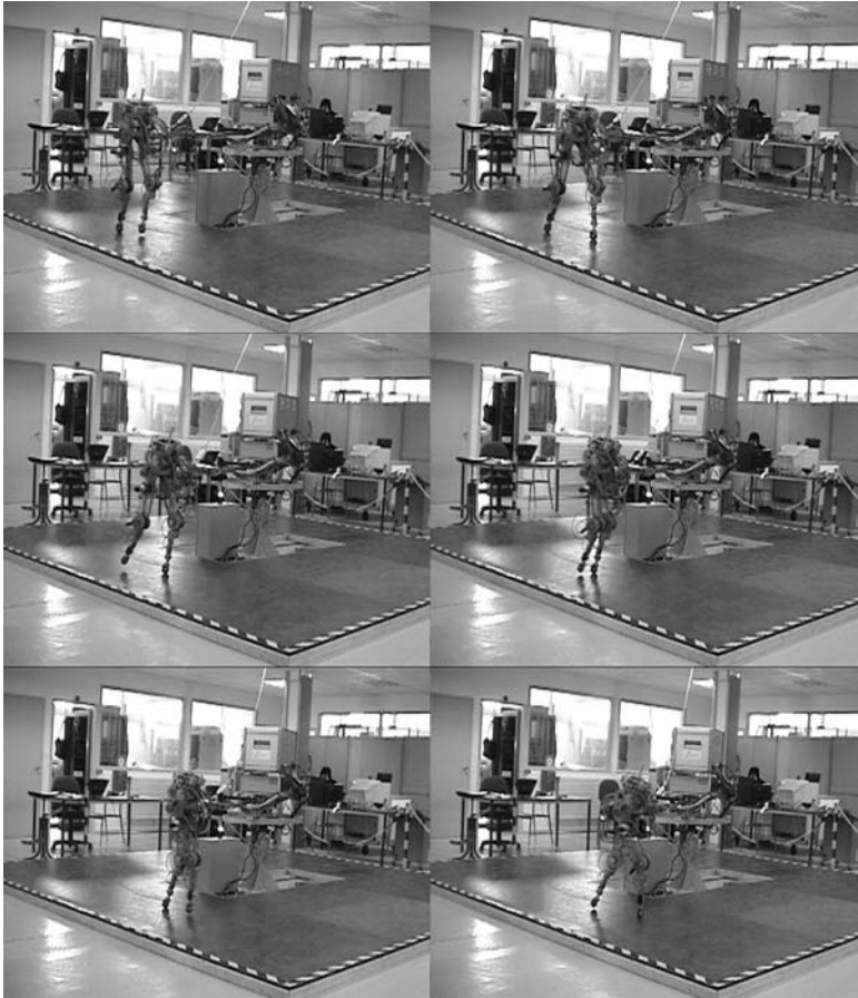
Figure 8.6. Video frames of RABBIT taking a step. The interval between frames is 120 ms. Note the safety cable attached to the boom to provide a measure of safety.
