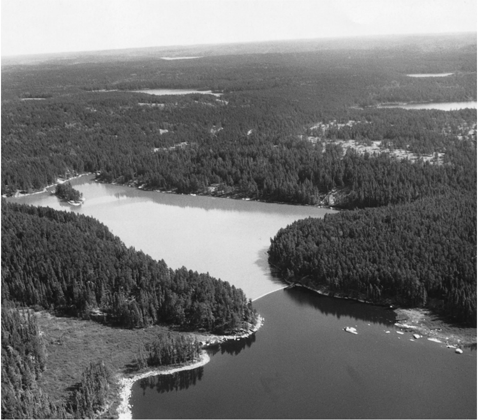
Plate 4.1 Whole-system manipulation illustrating the role of phosphorus in eutrophication. Legend: Lake 226, Experimental Lakes area, Ontario, Canada, was manipulated to address the role of phosphorus, nitrogen, and carbon respectively, in eutrophication. At the time, there was still considerable controversy about the effectiveness of controlling phosphorus entering freshwater lakes (Schindler 1974). In 1973, the far basin in the photograph was fertilised with phosphorus, nitrogen, and carbon and within two months was covered by an algal bloom (pale, solid area in the photograph). The near basin, which received similar quantities of nitrogen and carbon but no phosphorus, did not develop a bloom (dark, transparent area in the photograph). Photograph supplied by and reproduced by permission of David Schindler.
