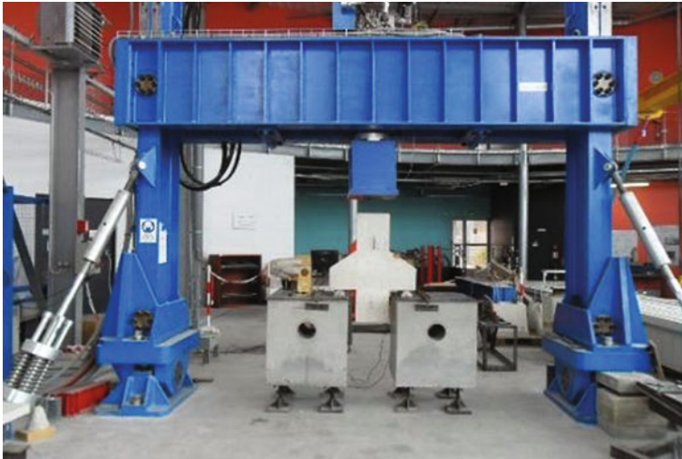
Fig. 14 Bending test machine with device of maximum to 1000 kN
