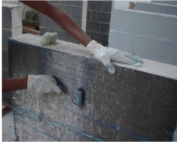
Fig. 6 Horizontal direction of the fibres in the wallettes. Source Chagas (2005)
