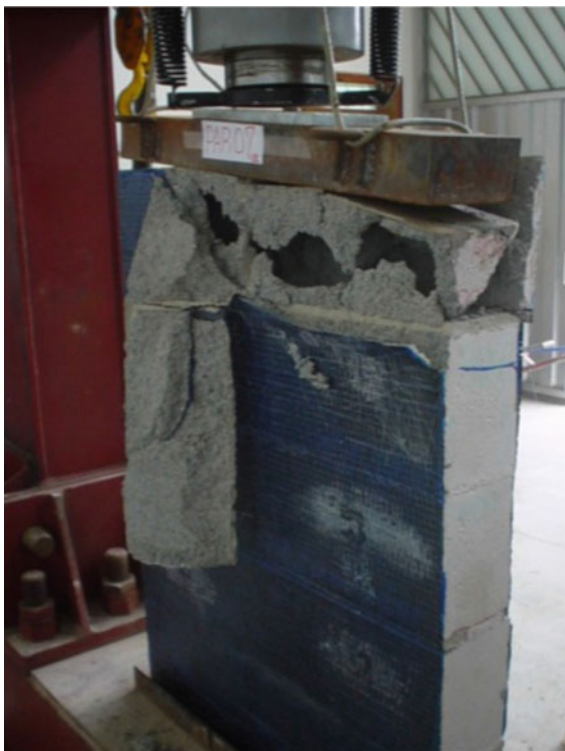
Fig. 11 Failure of the CW1 wallette reinforced with CFRP (without putty). Source Chagas (2005)
