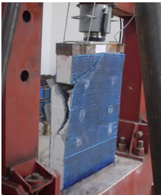
Fig. 9 Failure of the CW2 wallette reinforced with CFRP (with putty). a Frontal view and b lateral view. Source Chagas (2005)
