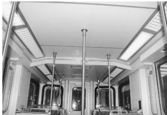
Figure 23-14. This train is lit with luminaires that have baffles to cut down on glare. The luminaires have been designed with passenger safety in mind.
