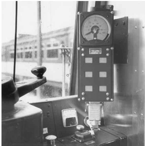
Figure 23-23. In this type of rapid transit cab signal, lighted segments on the speedometer show the highest speed permitted. The six windows below the speedometer light to show yellow, green, and red aspects and speed limits.
