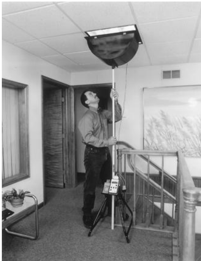
Figure 28-2. A fluxometer developed to measure a luminaire's available light in order to determine the benefits of periodic cleaning.
