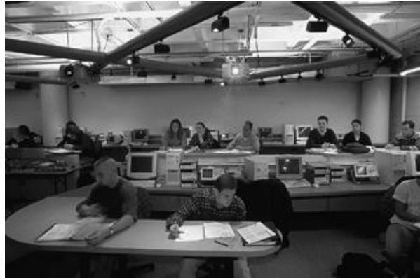
Figure 12-9. A lecture hall/interactive classroom outfitted with equipment for audiovisual presentations and student computers. Uplighting provides ambient lighting, while track lighting puts light on desk tops.
