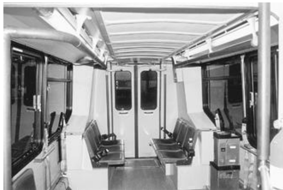
Figure 23-9. Interior of twelve-passenger paratransit vehicle, equipped with a lift to accommodate wheelchairs. Ceiling-mounted fluorescent luminaires provide diffuse semidirect illumination.
