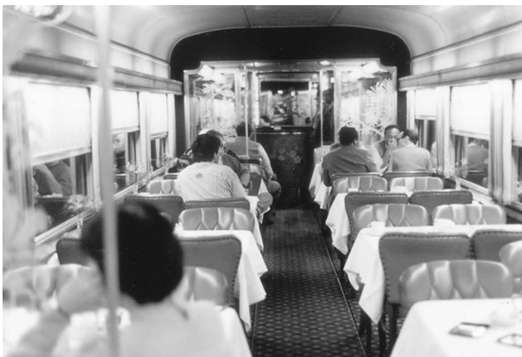
Figure 23-19. Well-controlled, diffuse lighting provides a comfortable, relaxing environment for dining. Low-glare incandescent point sources directed onto the table would add sparkle to enhance the visual environment.
