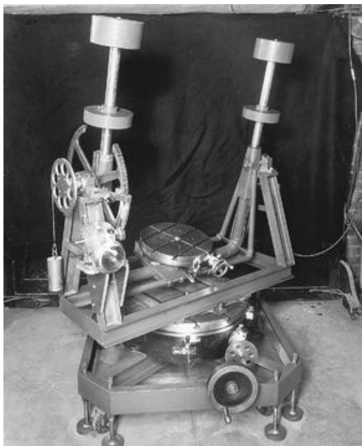
Figure 2-21. Typical goniometer for indoor photometric range. Two rotary tables of the type used in large machine tools are incorporated into the goniometer to provide two of the three rotations available. For horizontal distributions either the rotary table on which the outer frame is mounted or the inner table on which the test equipment is mounted may be used. This makes for flexibility and is especially useful for obtaining polar angle distributions. The inner frame with the test unit mounted can then be balanced with the adjustable counterweights. After balancing, a small constant torque is applied to the inner frame through the use of the pulley and weight at the side, thus eliminating backlash.
