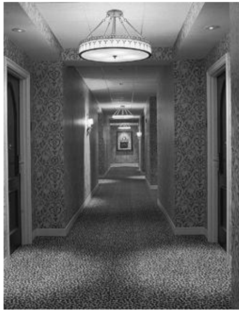
Figure 13-6. Corridor lighting should be designed to make hotel guests feel safe on their way to and from their rooms. Uplighting and spotlights on the carpet create visual interest, and at the same time provide adequate general light for passage and identifying room numbers and locks.
