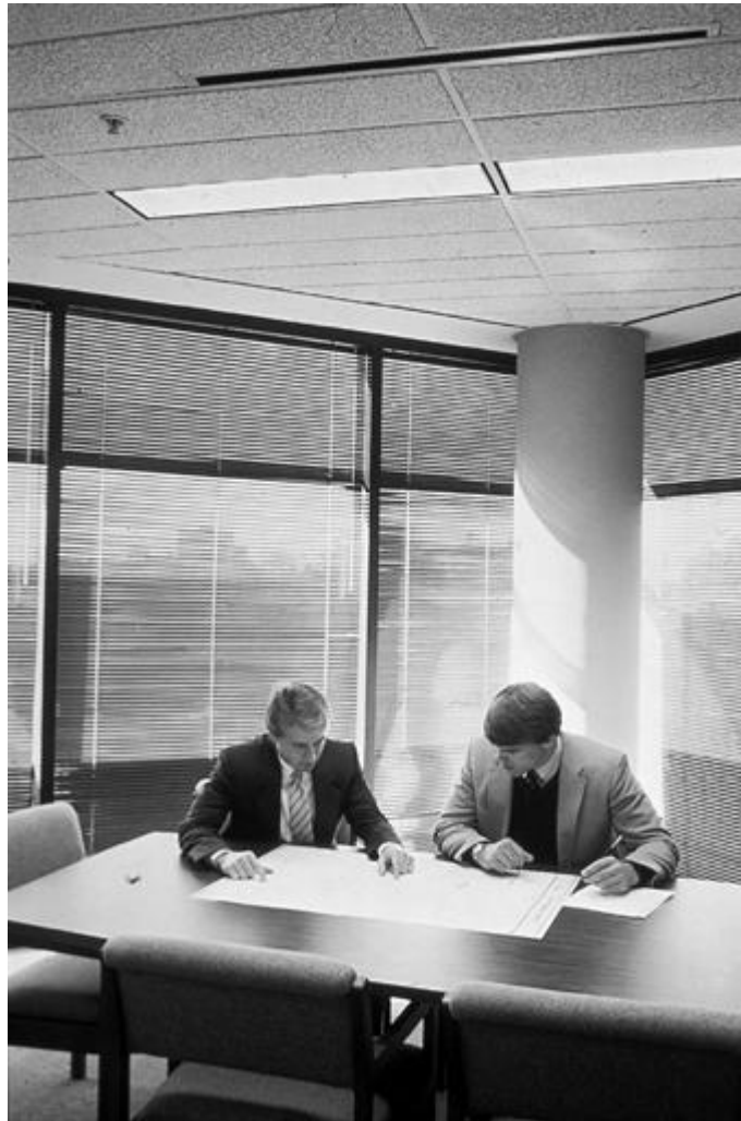
Figure 26-2. Effective utilization of daylight is important. Glare from fenestration should be controlled to the same degree as glare from luminaires.
