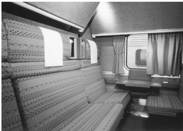
Figure 23-20. Sleeping car illuminated with a ceiling-mounted luminaire for general lighting and individually controlled beam-type lights for reading.
