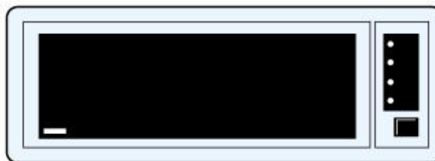
Figure 27-6. Example of multichannel preset station that provides four scenes of control for twelve
