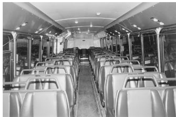
Figure 23-10. Intercity bus. Individually controlled beam-type incandescent lights are mounted over the seats to provide each passenger with a reading light.
