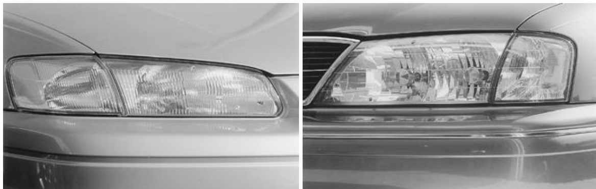
Figure 23-1. Headlight systems. (a) Parabolic reflector system, and (b) non-parabolic reflector system.
