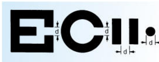
Figure 3-25. Commonly used test objects for determining resolution limits and visual acuity. The critical size is represented by the dimension d .
