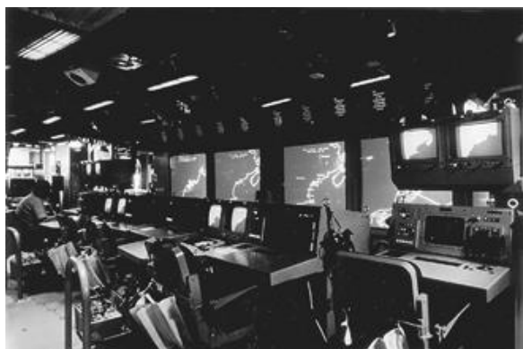
Figure 23-30. Low light levels in the combat information center of the U.S.S. Shiloh permit the viewing of visual displays and radar screens.
