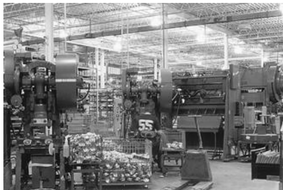
Figure 19-26. Widespread HID luminaires provide improved vertical luminance on the interior portions of the press to allow the operator to more accurately see the task.
