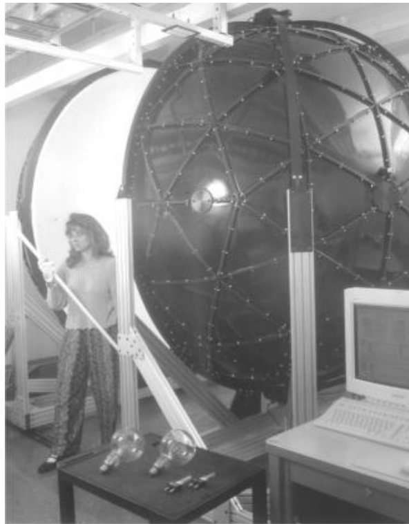
Figure 2-15. Ulbricht-type integrating sphere with diffuse high-reflectance coating, shown here at the National Institute of Standards and Technology (NIST).
