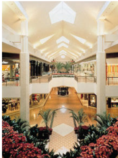
Plate 8. Shoppers use mall areas to rest and congregate. Lighting must address a variety of purposes: provide general ambient lighting; add emphasis where appropriate, yet not compete with individual store windows and entrances; and be flexible to accommodate special displays and attractions. Landscape lighting adds aesthetic beauty and serenity, and contributes to a desired image.
