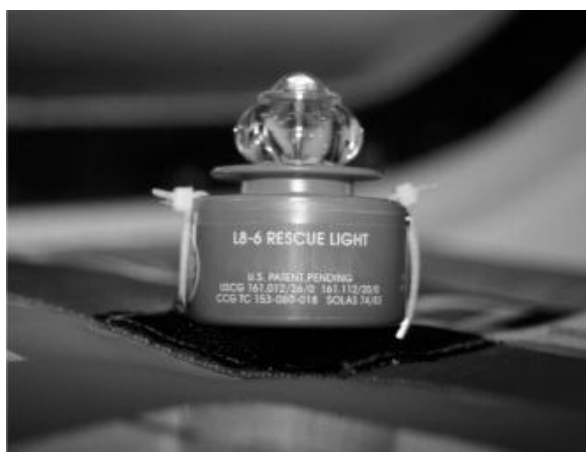
Figure 23-38. Rescue light mounted to a life vest. The light illuminates on impact with salt water.
