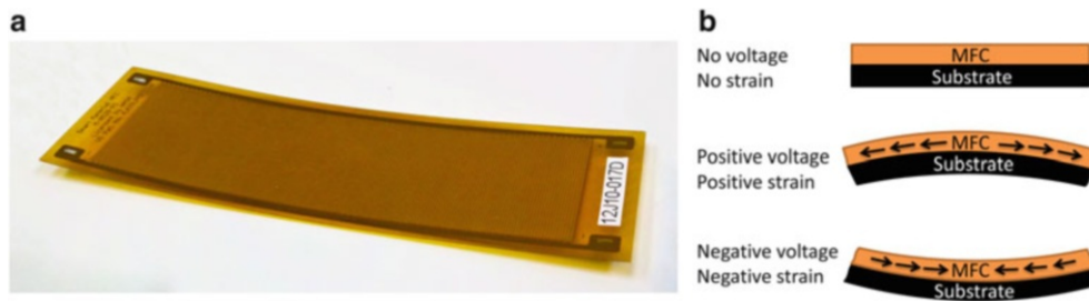
Fig. 12.1 (a) The M8528-P1 actuator fabricated by smart Materials Corporation with an active area measuring 85 mm by 28 mm (b) an illustration of the resulting curvature when adhering the MFC to a substrate
