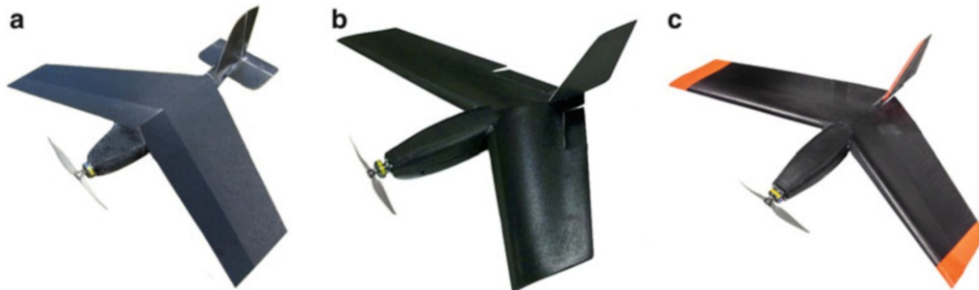
Fig. 12.15 (a) First iteration of forward swept wing with servo actuated tail surfaces. (b) Second iteration of forward swept wing with servo actuated elevons on the trailing edge of the wing. (c) Third iteration of forward swept wing with exclusive actuation provided by MFC actuators
