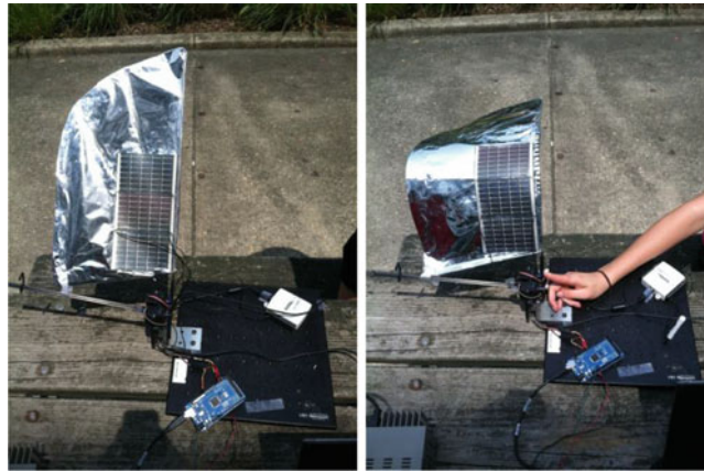
Fig. 10.8 Test setup for solar cells under full sunlight. Regular wing is shown on the left and compliant wing is shown on the right
