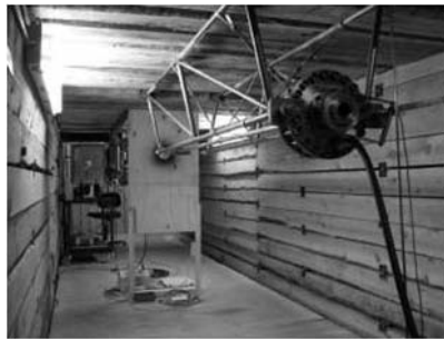
FIGURE 1. Compressed air gun with pressure chamber in the foreground, a box for a high speed camera and the rig for the kinematic pendulum can be seen in the background.
