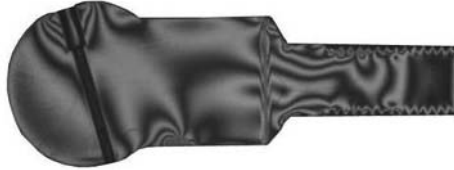
FIGURE 1. Dark field isochromatics captured using monochromatic light source
