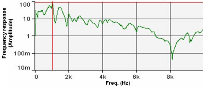
FIGURE 1. Response spectrum of FLD beam (test specimen 1)
