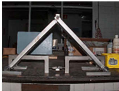
FIGURE 1. Experimental set-up for testing in liquid Zn.
