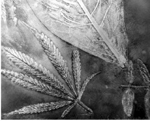
FIGURE 2: An example of a blast-embossed macro-structure (Source: Fraunhofer ICT)
