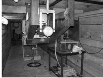
FIGURE 2. Rig for mounting test specimens and kinematic pendulum, with a box for mounting high speed camera to the left.
