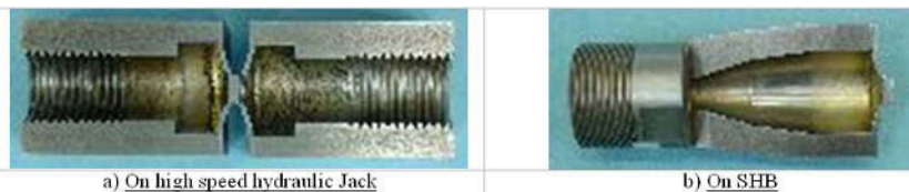
FIGURE 1. Shape of failed spotweld after tensile test
