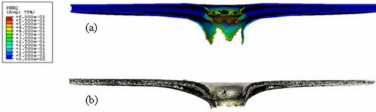
FIGURE 2: (a) Equivalent plastic strain contours for a sandwich panel impacted at 235 \text{ m s}^{-1} and (b) a photograph showing the equivalent experimental result.
