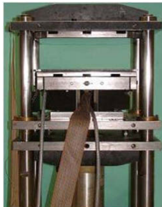
FIGURE 1. PIERS (Permeability Identification using Electrical Resistance Sensors) set-up.
