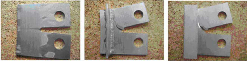
FIGURE 2. Unstiffened (left) and I-type welded (middle) and T-type extruded (right) CT specimens tested under varied displacement rate
