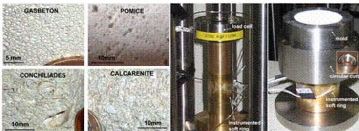
FIGURE 1. High porosity soft rocks tested and the Soft Oedometer Apparatus
