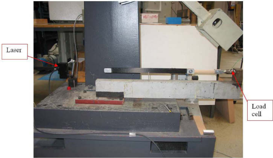
FIGURE 1. Test setup for strain rate testing. The raised pendulum connects with the stiff carbon fiber rod when vertical, bringing the rod and one end of the specimen with it. The other end of the specimen is locked in a small aluminum fork connected directly to the load cell. The laser keeps track of the pendulum position and the pendulum speed can be calculated.
