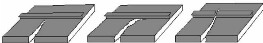
FIGURE 1. A conceptual sketch of the crack arrestor. Stopping the crack (left), redirecting (center), and passing through (right)
