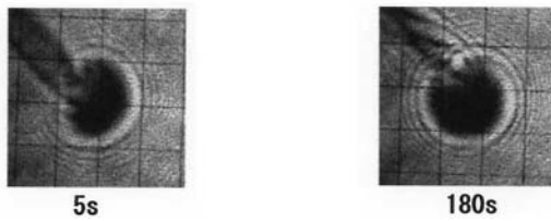
FIGURE 3. Example of caustic patterns for glass plate with an inclined notch at 673K by convergent light ( \theta = 45^\circ )
