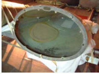
FIGURE 1. The repaired composite sandwich structure
