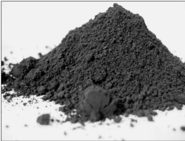
Figure 3.2-5. Rice husk ash ground to 9 \mu\text{m} . (Meryman 2007)
