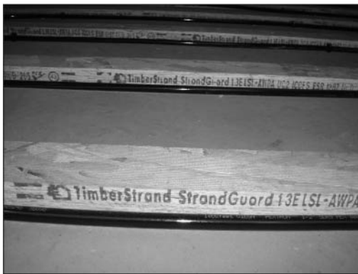
Figure 3.5-9. Borate treatment is an effective non-toxic preservative. (Photo by DeStefano & Chamberlain, used with permission)
