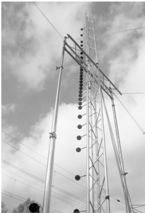
Fig. 5.13 Vertical linear microphone array applied in the pass-by noise measurement of rail vehicles
