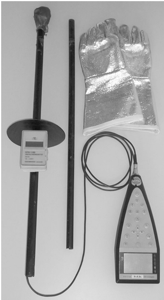
Fig. 5.18 This heat-protected microphone probe (with hand heat shield, on-board thermometer and extension rod) is equipped with a standard ½-inch condenser microphone and is suited for short-term measurements inside flue gas ducts or similar piping with gas temperatures up to 600°C
