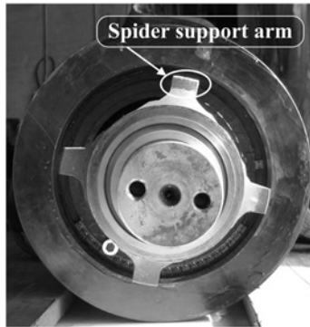
Figure 9.4 Rotor shaft to show spider support arms (4 of) and axial cooling ducts (4 of).
