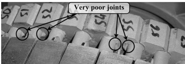
Figure 5.16 Visual inspection after cleaning and prior to NDT dye penetrant test.
