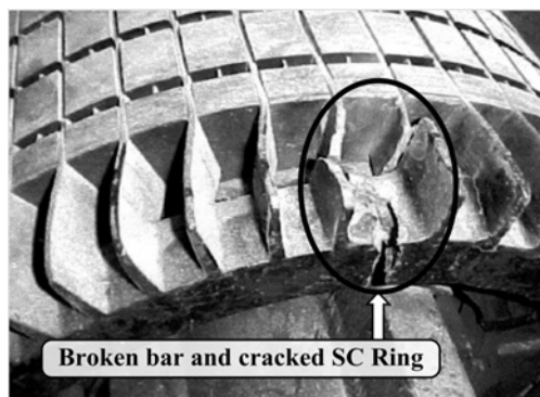
Figure 3.18 Fabricated copper cage winding with breaks in bars and end ring. Reproduced with permission of EASA, USA.
