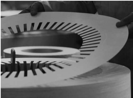
Figure 1.24 Stator core laminations. Reproduced with permission of Parsons Peebles, Scotland.
