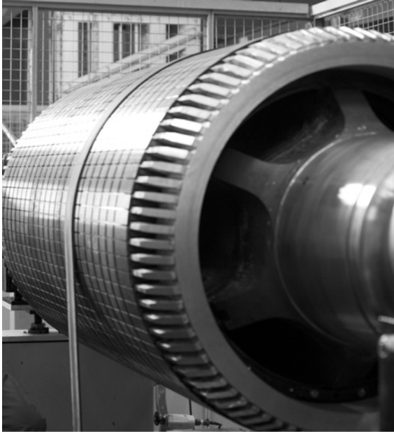
Figure 1.25 Squirrel cage rotor. Reproduced with permission of Parsons Peebles, Scotland.
