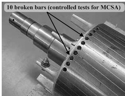
Figure 4.18 The 51 slot aluminum die-cast rotor with 10 broken rotor bars.
