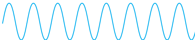
(b) The sound wave generated by a tuning fork vibrating at 880 vibrations per second [This note is an A one octave above that in part (a).]
