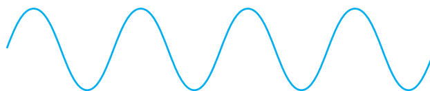
(a) The sound wave generated by a tuning fork vibrating at 440 vibrations per second (On the piano, this note corresponds to the first A above middle C.)
