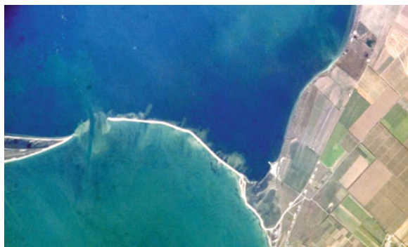
Photo 7.14 After construction of dam in 2003, width of the Tuzla channel does not exceed 300 m (photo from ISS)
