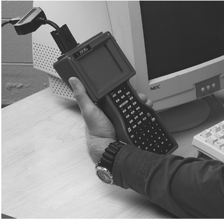
FIGURE 1-15. Tripod Data Systems' Ranger data collector. (Courtesy of Tripod Data Systems, Inc.)
