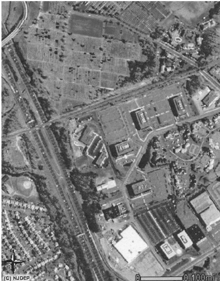
FIGURE 1-3. Practically every line recorded on this photograph was laid out with a transit, a steel tape, and a level—the primary equipment of the surveyor. (Courtesy of New Jersey Department of Environmental Protection)
