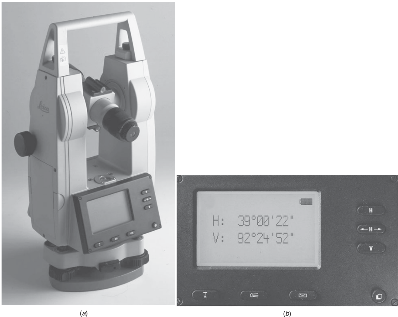
FIGURE 6-25. (a) An electronic digital theodolite. (b) Digital display of horizontal angle = 39^{\circ}00'22'' and vertical angle = 92^{\circ}24'52'' . (Courtesy of Leica Geosystems, Inc.)
