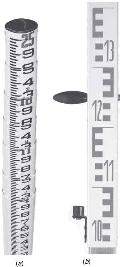
FIGURE 5-14. (a) Telescoping fiberglass rod. (Courtesy of Sokkia Corporation.) (b) Polymer bar-coded staff. (Courtesy of Leica Geosystems, Inc.)
