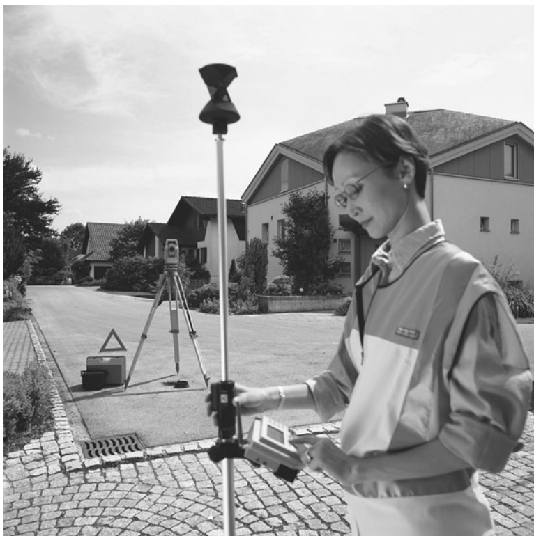
FIGURE 1-16. One-person crew using a robotic instrument and data recorder. (Courtesy Leica Geosystems, Inc.)
