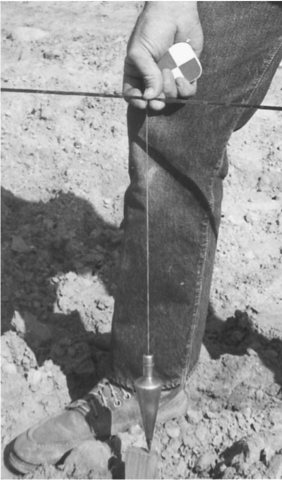
FIGURE 4-7. A plumb bob is one of the simplest yet most important accessories for accurate surveying. The vertical cord transfers a position from the steel tape to the wooden stake in the ground. (Courtesy of The Lietz Company)
