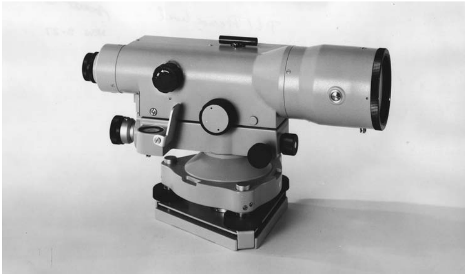
FIGURE 5-23. A precise level with parallel plate micrometer enables vertical displacement to be measured to 0.1 mm. An accuracy of \pm 0.2 mm in 1 km of leveling ( \pm 0.001 ft/ml) can be obtained. (Courtesy of The Lietz Company.)
