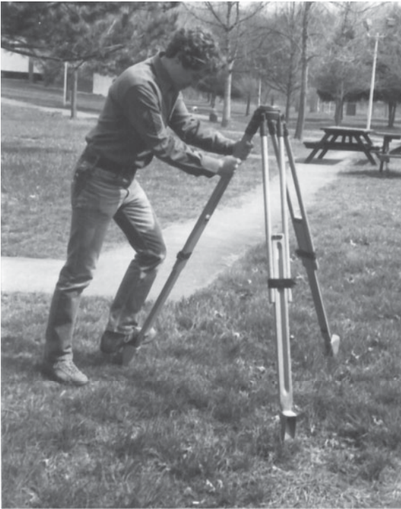
FIGURE 5-16. The pointed metal shoe at the end of each tripod leg must be pressed firmly into the ground.
