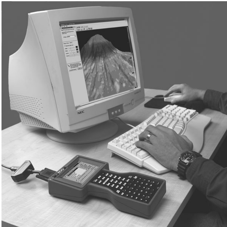
FIGURE 1-17. An electronic field book that collects and stores information from surveying instruments; notes that identify stations can also be entered or displayed. The stored information can be “dumped” into an office computer for computations. (Courtesy of Tripod Data Systems, Inc.)
