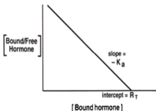
Figure 37.3. Diagram of Scatchard analysis, showing the relationship of slope to -K_a and of the intercept to the total number of receptors.
