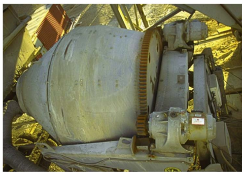
The work of the torque or moment developed by the driving gears on the motors is transformed into kinetic energy of rotation of the drum.
