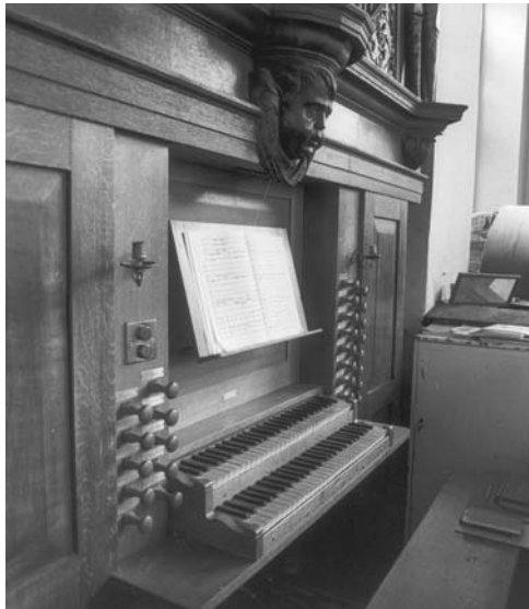
Figure 19.2 Close-up of the organ loft, showing the two keyboards, or "manuals". The wooden knobs on either side of the manuals are the stops. The pedalboard is out of sight below the bench.
