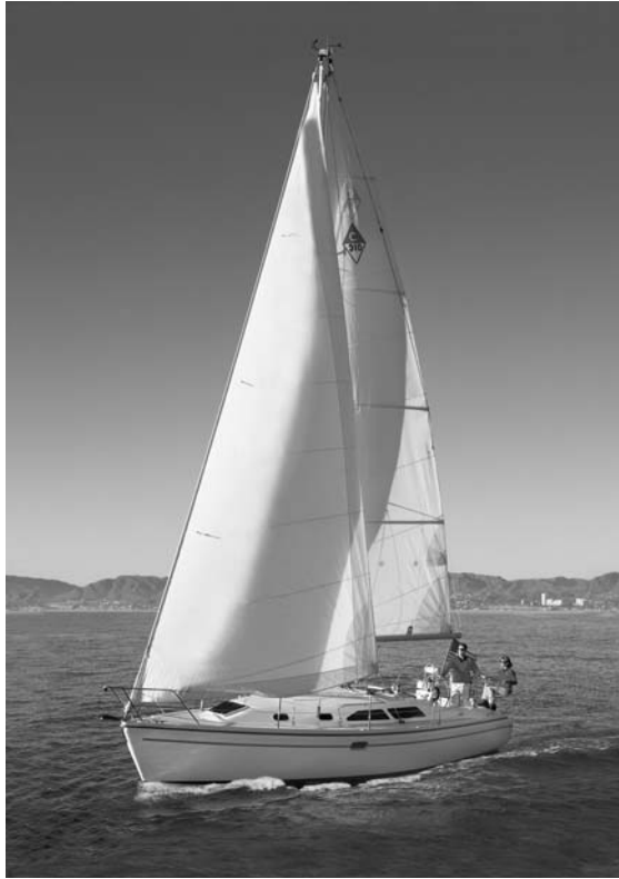
Figure 1.5 A sailing cruiser, with composite (GFRP) hull, aluminum alloy mast and sails made from synthetic polymer fibers.
