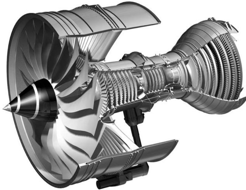
Figure 1.3 Cross-section through a typical turbofan aero-engine.
