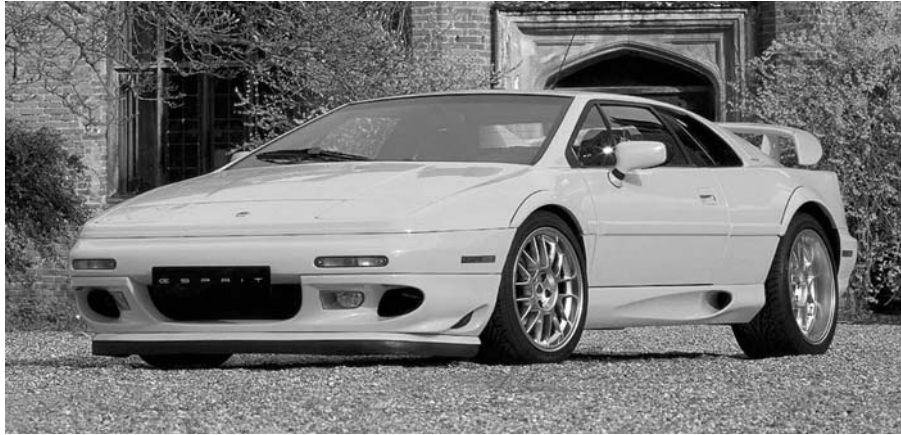
Figure 31.7 A Lotus Esprit, with a GFRP body (but still mounted on a steel chassis — which does not give anything like the weight saving expected with an all-GFRP monocoque structure).
