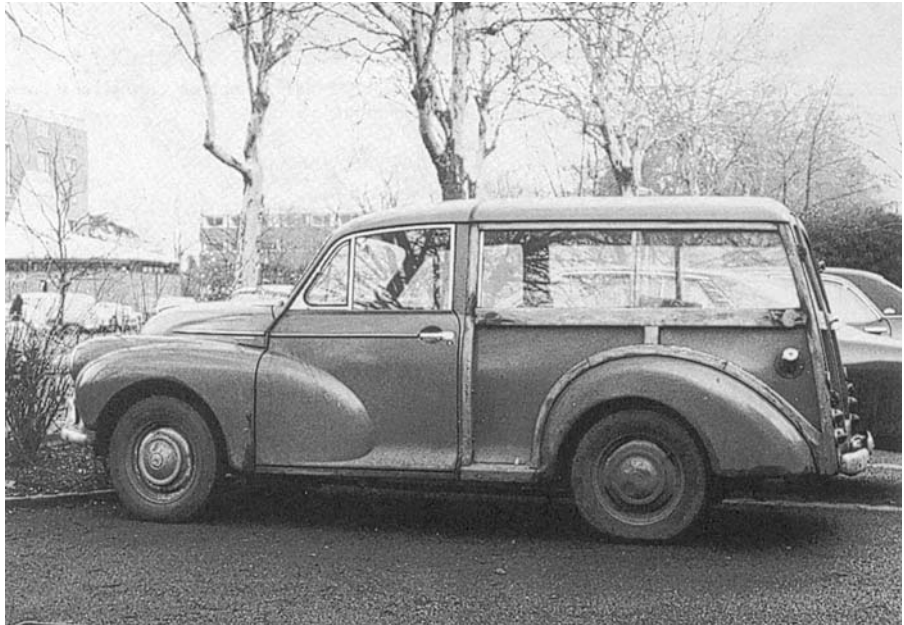
Figure 31.3 The Morris Traveller — a classic of the 1950s with wooden members used as an integral part of the monocoque body shell.
