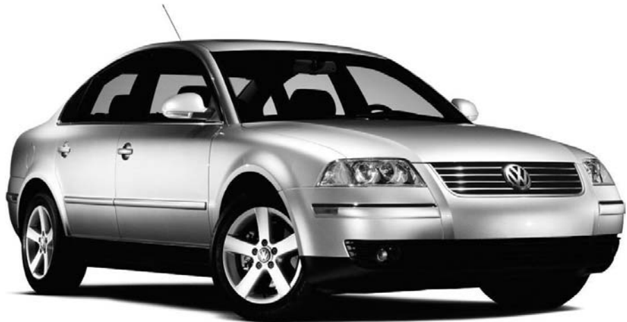
Figure 31.2 The Volkswagen Passat — a typical modern pressed-steel body with no separate chassis. For a given material this “monocoque” construction gives a minimum weight-to-strength ratio.
