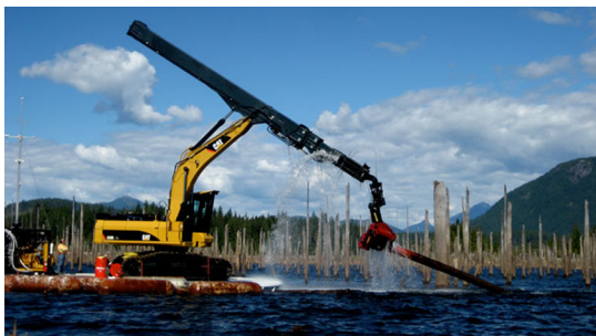
Figure 7. Triton “sharc” underwater harvester (Triton Logging, 2012)
