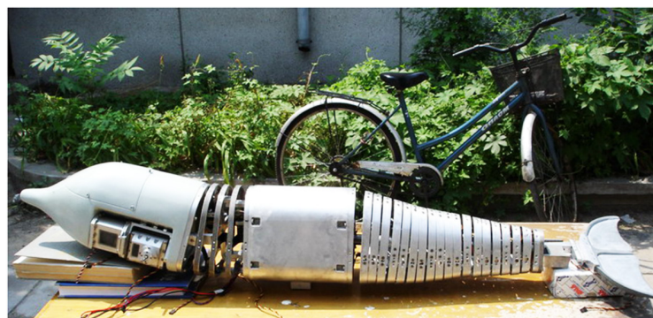
Figure 7. Uncoated dolphin robot built by Yu et al. (2007).
