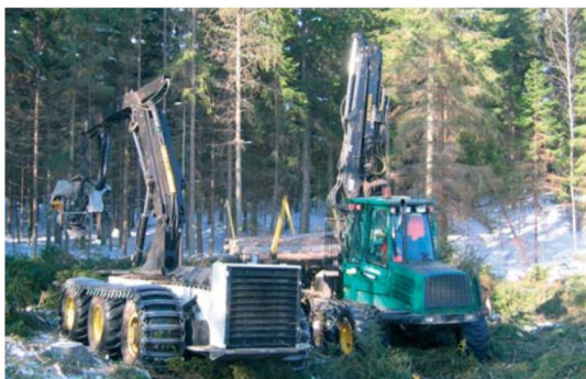
Figure 6. "Besten" remote controlled harvester. Forwarder on right (Bergkvist, Nordén, et al., 2006).
