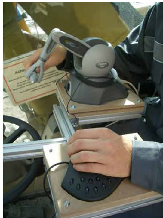
Figure 24. Excavator teleoperation with haptic feedback (Hayn & Schwarzm ann, 2010)
