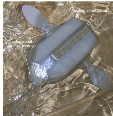
Figure 8. MARCO inspired by a boxfish as an ostraciiform (Kodati, et al., 2008)
