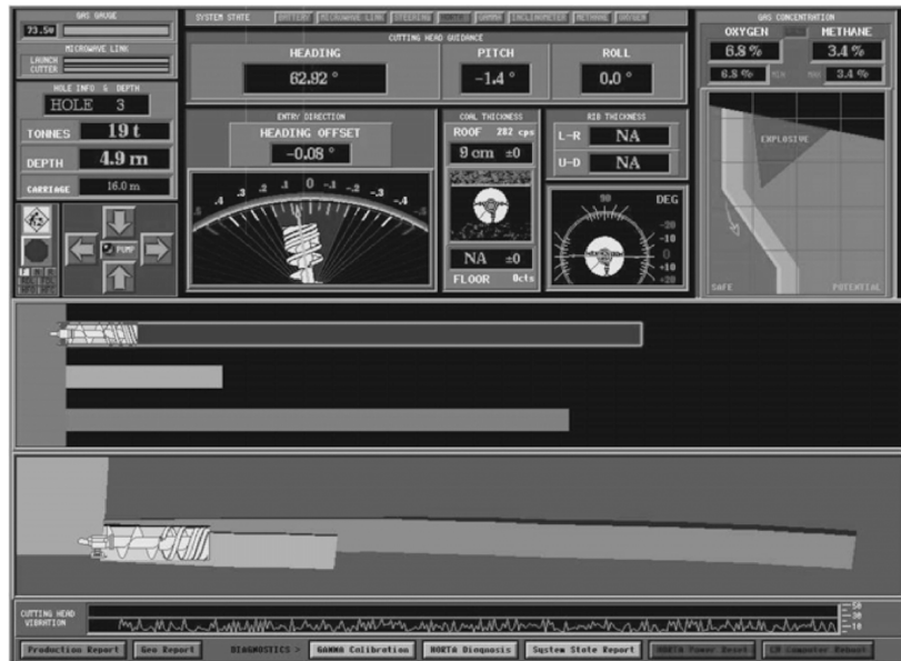
Figure 12. High wall coal miner status screen (Hainsworth, 2001)
