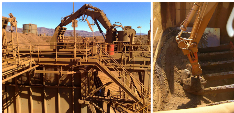
Figure 10. Teleoperated ore crusher (Duff, Caris, et al., 2009; Zhu, Gedeon, et al., 2011)
