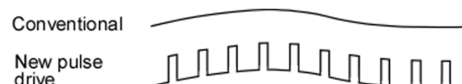
Figure 15. Pulse steering drive method, compared with conventional drive method (Wakaumi, Nakamura, & Matsumura, 1989)
