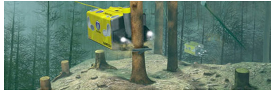
Figure 8. Triton “sawfish” underwater logging vehicle (Triton Logging, 2012)
