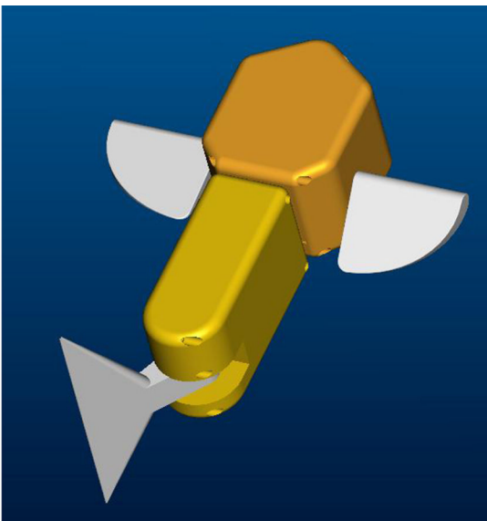
Figure 12. BoxyBot as a labriform-like and an ostraciiform-like robot (Lachat & Ijspeert, 2005)
