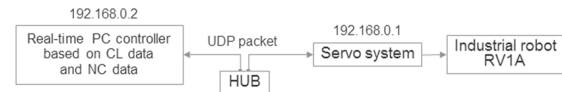
Figure 6. Block diagram of communication system by using UDP packet between a PC and an industrial robot RV1A
