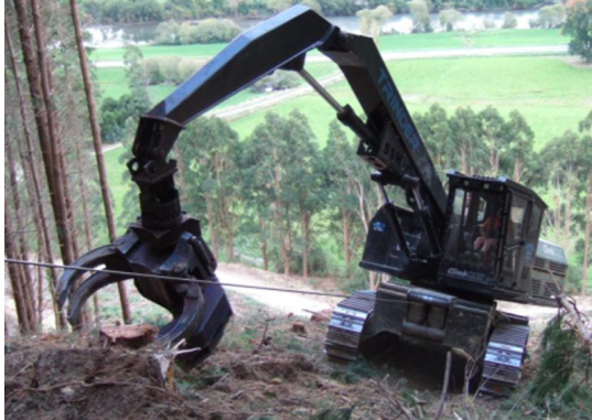
Figure 1. Trinder ClimMAX winch harvester beta prototype (Evanson and Amishev, 2010; Raymond, 2012)
