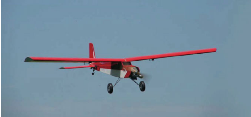
Fig. 21.1 Senior Telemaster for use as a UAS research platform
