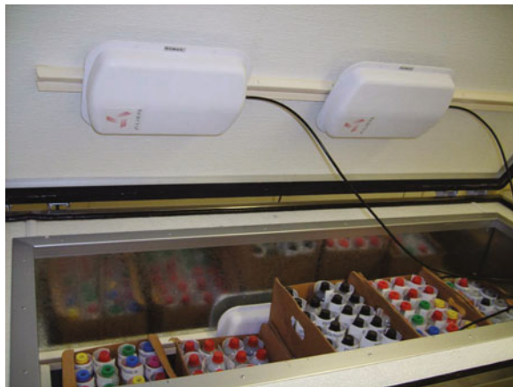
Fig. 48.4 RFID antenna locations for smart freezer solution
