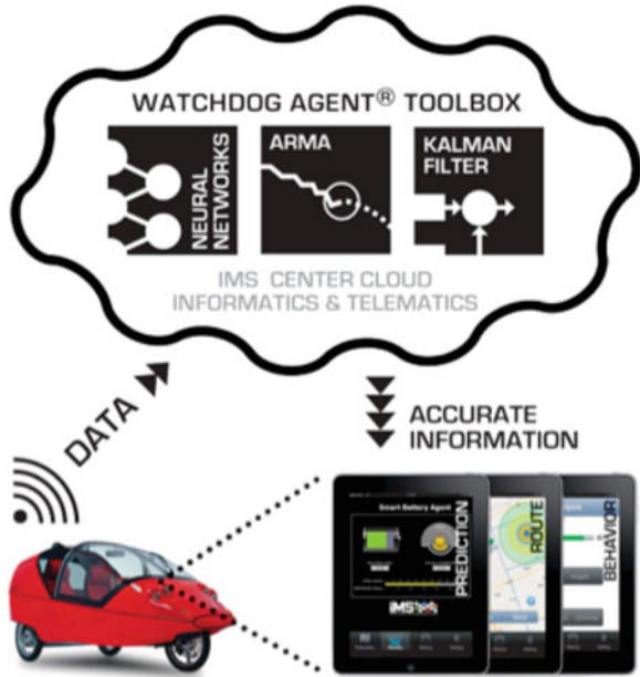
Fig. 22.7 Cloud-based informatics and telematics platform
