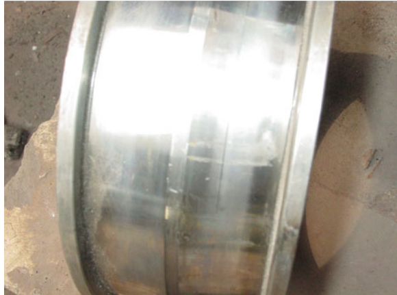
Fig. 27.12 A slight scratch on the inner-race of the bearing
