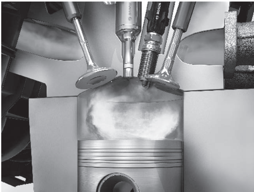
FIGURE 13.4.4 High-pressure-injection arrangement, Photo: Bosch.
