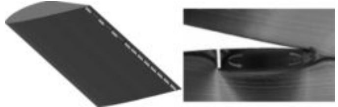
FIG. 7.31 MICROTAB ACTIVE AERO CONCEPT AND CFD CALCULATION
