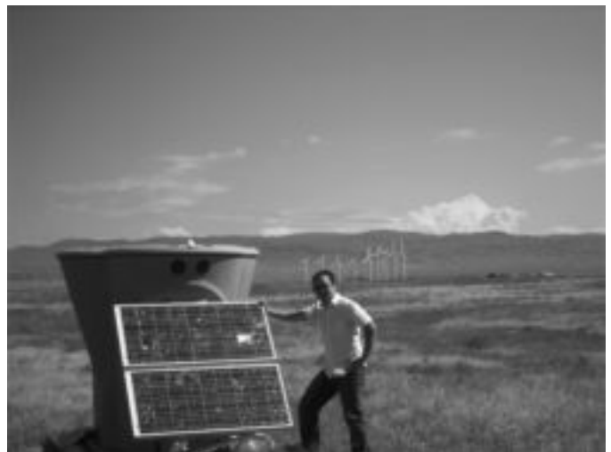
FIG. 8.14 BOISE STATE UNIVERSITY ENGINEERING STUDENT KEN FUKUMOTO STANDS NEXT TO A TRITON™ SODAR NEAR MOUNTAIN HOME, ID (Photo Courtesy of Todd Haynes, 2009)
