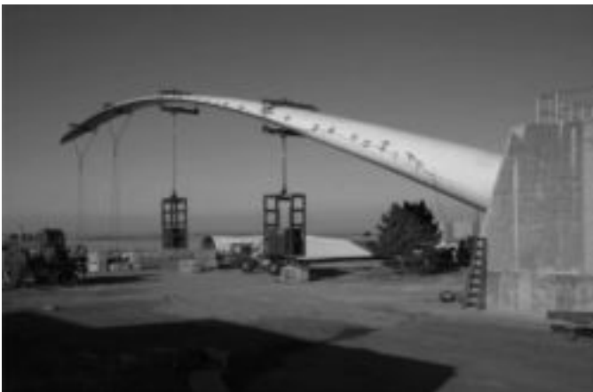
FIG. 7.26 UTILITY SCALE STATIC TESTING AT NREL'S NWTC
