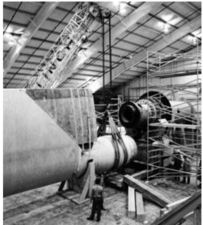
FIG. 6.31 NASA'S BLADE TECHNOLOGY PROGRAM DEVELOPED 50 METER BLADES USING AUTOMATED MANUFACTURING TECHNIQUES THAT COULD BE ADOPTED TODAY
