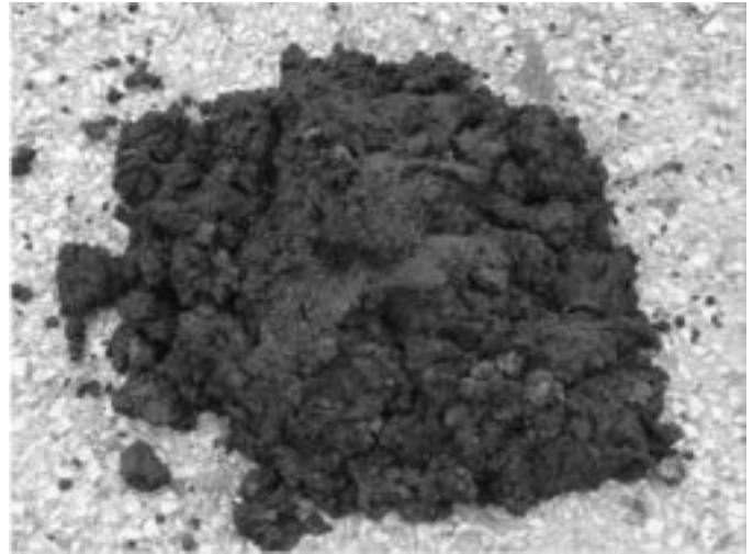
SEWER SLUDGE (30% Solids and 70% Moisture)
