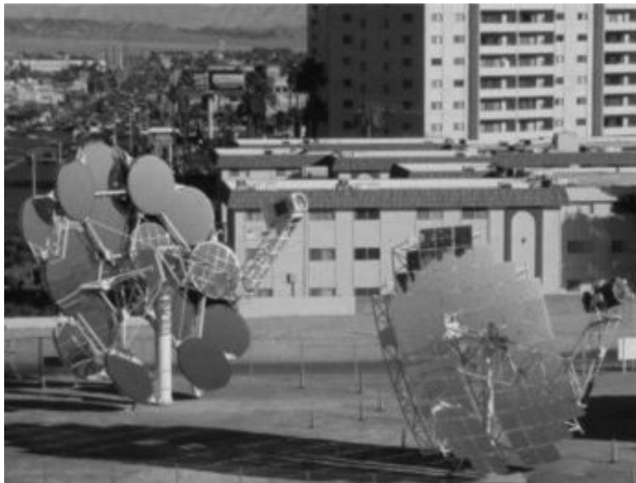
FIG. 1.8 TWO DIFFERENT DESIGNS OF DISH-STIRLING SOLAR DEVICES ARE SHOWN ON THE UNIVERSITY OF NEVADA, LAS VEGAS (UNLV) CAMPUS IN THE EARLY 2000S. THE UNIT ON THE RIGHT IS A DESIGN OWNED BY SES AND ON THE LEFT IS A DESIGN FROM SAIC INTERNATIONAL (Courtesy of UNLV)
