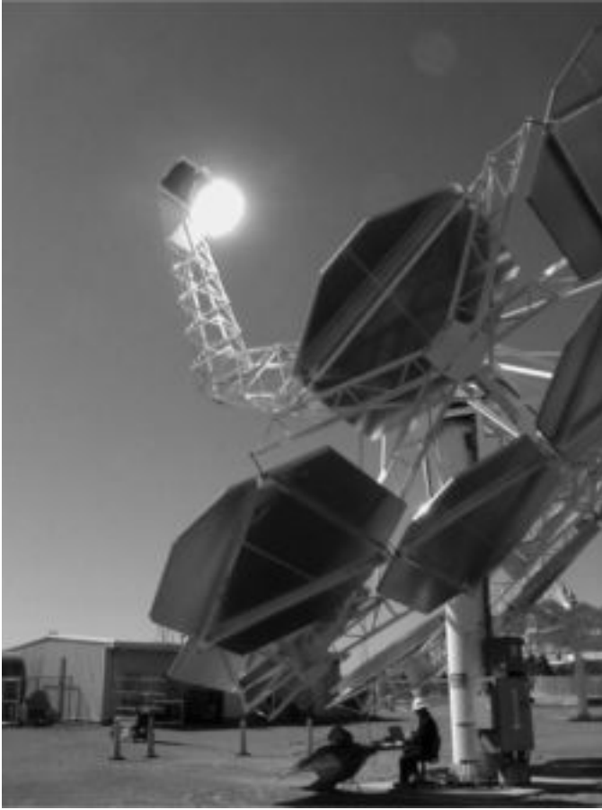
FIG. 1.12 A DISH-PV CONCENTRATING SYSTEM IS SHOWN OPERATING ON SUN. THE CONCENTRATION IS APPROXIMATELY 250X (From UNLV)
