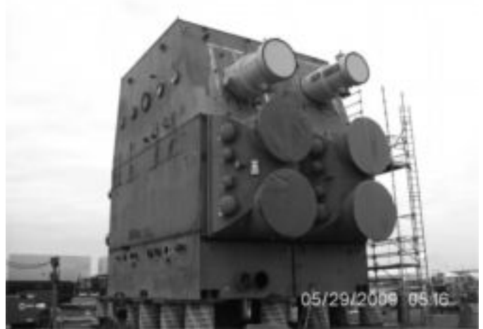
PHOTOGRAPH A: A TWO-TUBE PASS RECTANGULAR 900MW SUPERCRITICAL COAL-FIRED PLANT (Courtesy Holtec International)
