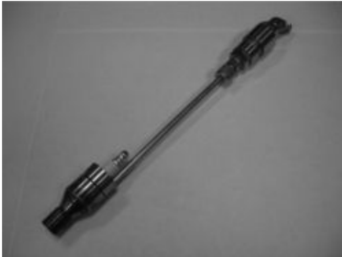
FIG. 1.16 AN INTEGRAL IN CYLINDER FUEL INJECTOR AND SPARK PLUG ASSEMBLY IS SHOWN. THIS ASSEMBLY REPLACES THE CONVENTIONAL SPARK PLUG OF A CONVENTIONAL SPARK IGNITION ENGINE [18]
