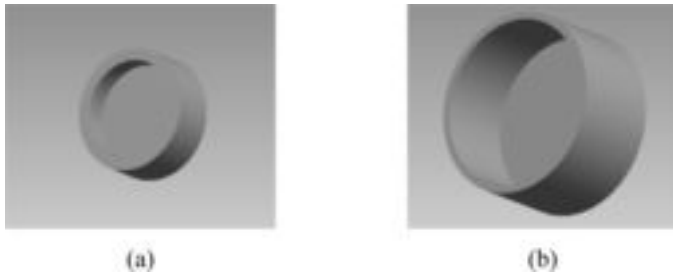
FIG. 31.6 TWO DIFFERENT PARTS WITH EQUAL VOLUME BUT DIFFERENT WALL THICKNESSES AND COOLING TIMES. PART (A) HAS A WALL THICKNESS OF 1.27 MM, WHILE PART (B) HAS A WALL THICKNESS OF 0.635 MM. BOTH PARTS HAVE A VOLUME OF 54.7327 CM 3
