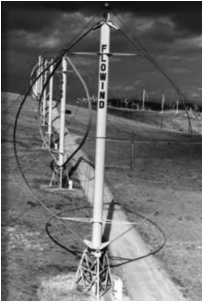
FIG. 7.5 FLOWIND COMMERCIAL 19-m VAWT COMMERCIALIZED IN COOPERATION WITH SANDIA
