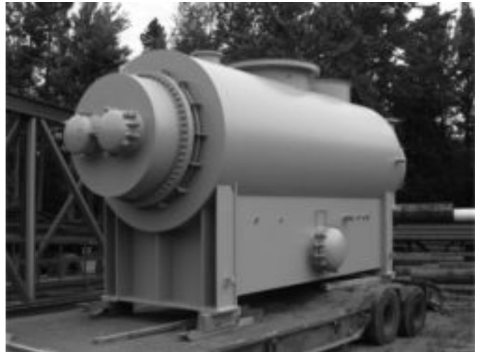
PHOTOGRAPH B: CONDENSER FOR 80MW COMBINED CYCLE PLANT (Courtesy Holtec International)
