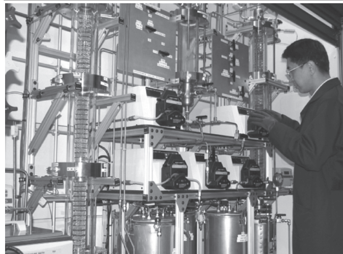
FIG. 18.18 BENCH-SCALE PCCC UNIT
