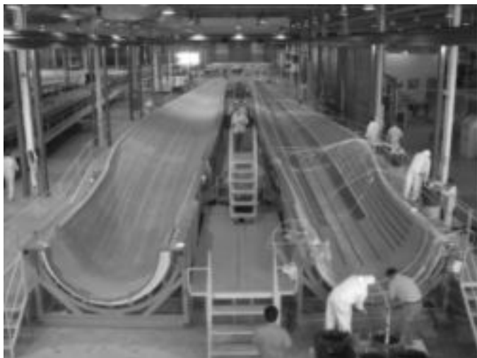
FIG. 7.11 PICTURE OF UTILITY SCALE BLADE MANUFACTURING (Courtesy of TPI)
