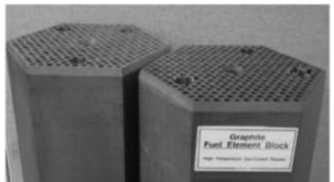
FIG. 23.24 GRAPHITE FUEL ELEMENT BLOCK FOR A PRISMATIC VHTR CORE [81]
