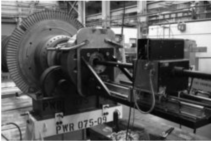
FIG. 25.3 BORESONIC DRIVE ATTACHED TO AN HP/IP ROTOR
