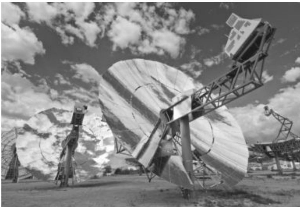
FIG. 1.9 UNITS OF A RECENT DESIGN OF THE SES DISH-STIRLING SYSTEM (THE SUNCATCHER™) ARE SHOWN HERE AT SANDIA LABORATORIES UNDERGOING EVALUATION (From SANDIA Laboratories)
