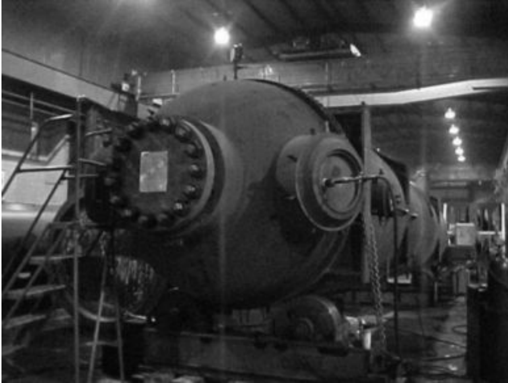
FIG. 29.5 THREE-ZONE, HIGH-PRESSURE, MANWAY ACCESS FEEDWATER HEATER UNDERGOING HYDROSTATIC TESTING [Photograph by MGT Inc., Boulder, CO During Shop Inspection]
