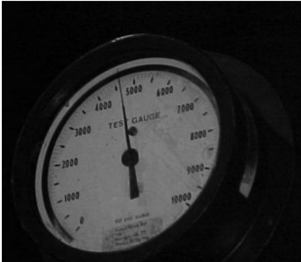
FIG. 29.7 TYPICAL BOURDON TUBE TEST GAGE USED IN TESTING HIGH PRESSURE FEEDWATER HEATERS [Photograph by MGT Inc., Boulder, CO During Shop Inspection]
