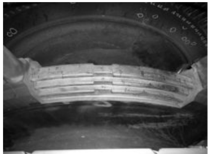
FIG. 25.12 STRADDLE-MOUNT, TANGENTIAL ENTRY BUCKETS AND RIM WITH LOADING NOTCH SHOWING
