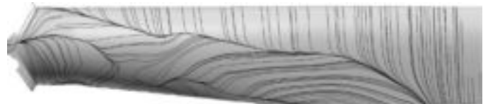
FIG. 7.20 CFD SOLUTION SHOWING NEAR-SURFACE FLOW STREAMLINES OVER THE INBOARD REGION OF A UTILITY-SCALE WIND TURBINE BLADE, SHOWING A REGION OF THREE-DIMENSIONAL SEPARATED FLOW
