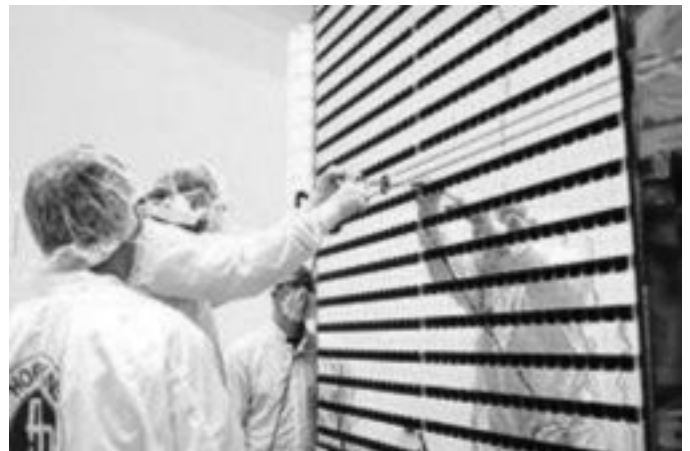
FIG. 6.15 SOLAR PANEL FOR THE MESSENGER MISSION TO MERCURY, SEEN IN THE ASSEMBLY PHASE. NOTE THE OPTICAL REFLECTORS COVERING MUCH OF THE SURFACE OF THE ARRAY
