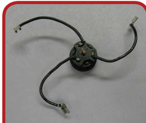
Three-phase overload for compressor. (Delmar/Cengage Learning)
