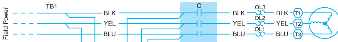
(a) Across-the-line starter (shaded area)
