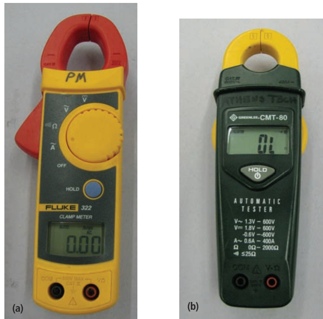
Digital clamp-on ammeters with volt-ohm functions. (Delmar/Cengage Learning)
