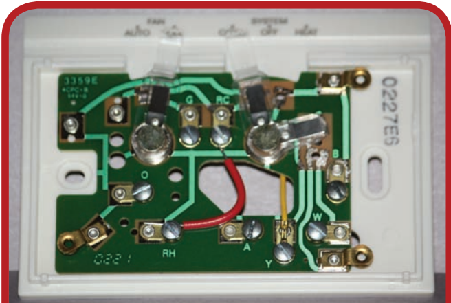
Common low-voltage thermostat subbase. (Delmar/Cengage Learning)
