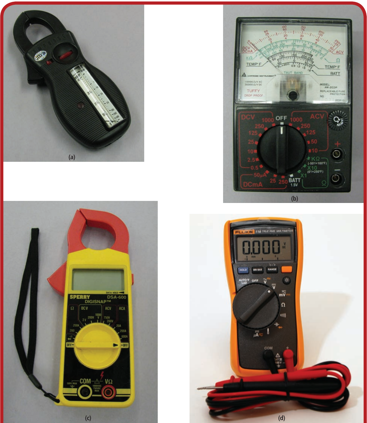
(a) Analog clamp-on ammeter with volt-ohm function (b) Analog volt-ohm meter (c) Digital clamp-on ammeter with volt-ohm function (d) Digital volt-ohm meter. (Delmar/Cengage Learning)
