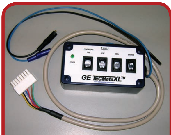
Electronic module used to troubleshoot ECM. (Delmar/Cengage Learning)
