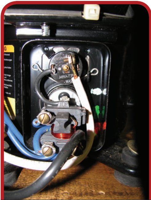
In-line overload on fractional horsepower compressor. (Courtesy of Tecumseh Products Co.)
