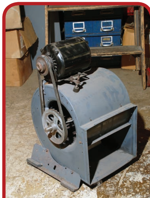
V-belt connection between fan and motor. (Delmar/ Cengage Learning)
