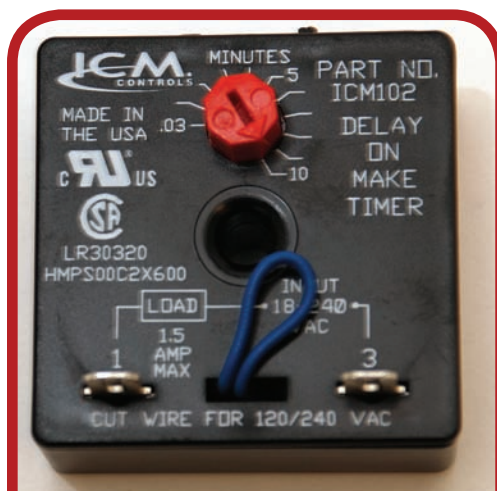
Electronic timer (delays close of contacts when energized). (Delmar/Cengage Learning)
