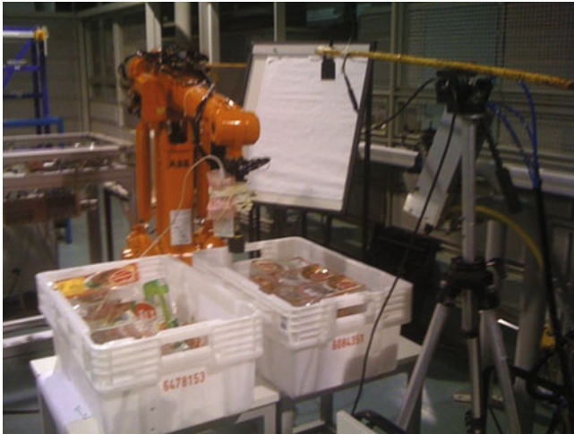
Fig. 85.2 Testing of the vision system applied on the autonomous packaging robot
