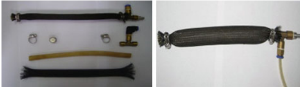
Fig. 208.2 Materials of PM actuator and PM actuator made in lab
