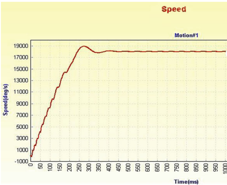
Fig. 234.9 Speed curves when the machine no-load running time is 1 s
