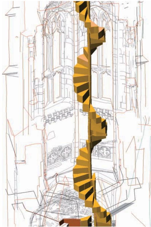
Figure 4.7 3D data collection for 3D model. The spiral stair has been solid modelled; the outline of all other features are in 3D wireframe. Views of the stair on the sectional elevation.
