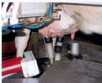
A three-teater: the front left quarter has been milked and the cup has been removed. Most robots remove each cup separately when the quarter is empty. As a result, there is very little over-milking and stress on the teats is minimised.
