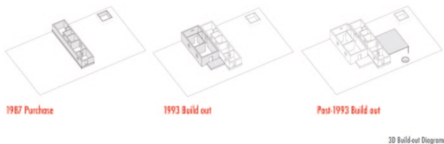
Fig. 15.1 Trailer and home extension build out, Las Lomas Colonia, Starr County
